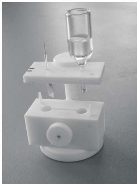
Fig. 1. Special spectroelectrochemical cell.
