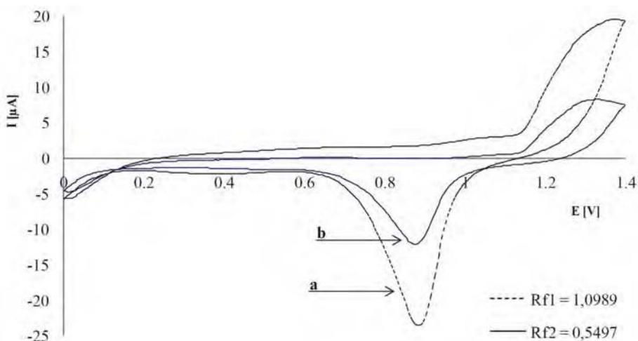
**Fig. 2** Cyclic voltammograms curves registered for bare gold electrode in 0.5 M  $\text{H}_2\text{SO}_4$  solution during electrochemical cleaning of electrode surface for (a) properly, and (b) improperly cleaned electrodes.
