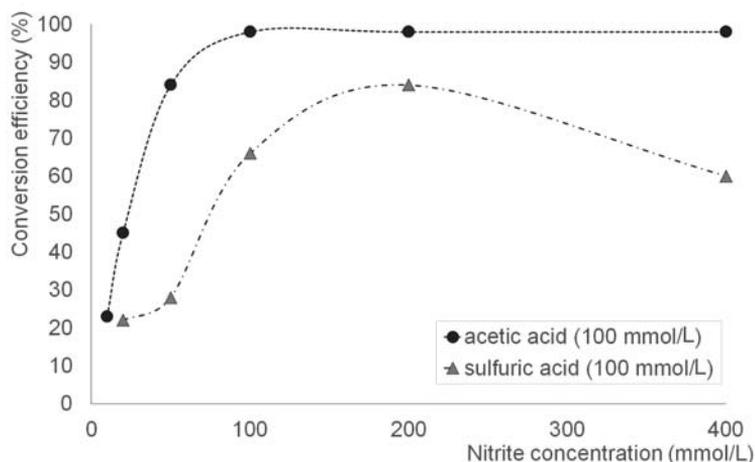
**Fig. 1** Dependence of leucine conversion efficiency on sodium nitrite concentration for acetic and sulfuric acid.
