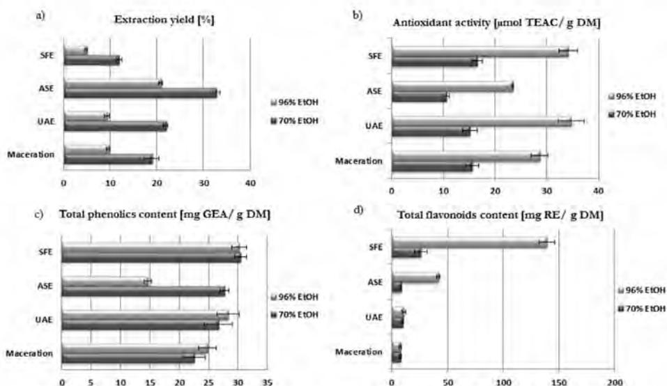
**Fig. 1** (a) Extraction yields, (b) antioxidant potential, (c) level of total phenolics content, and (d) total flavonoids content in *Medicago sativa* leaves extracts obtained with using different techniques of extraction.
