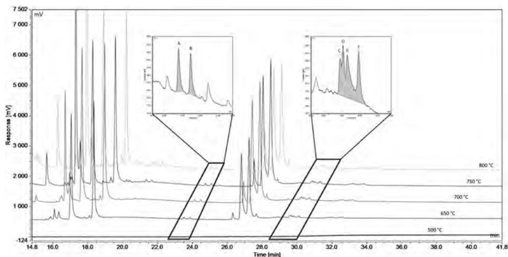
**Fig. 3** GC-NCD chromatogram of artificially bacterially contaminated (*Escherichia coli*) beer sample at different pyrolytic temperatures. Nitroso compounds produced by contamination are zoomed at pyrolytic temperature 750 °C.
