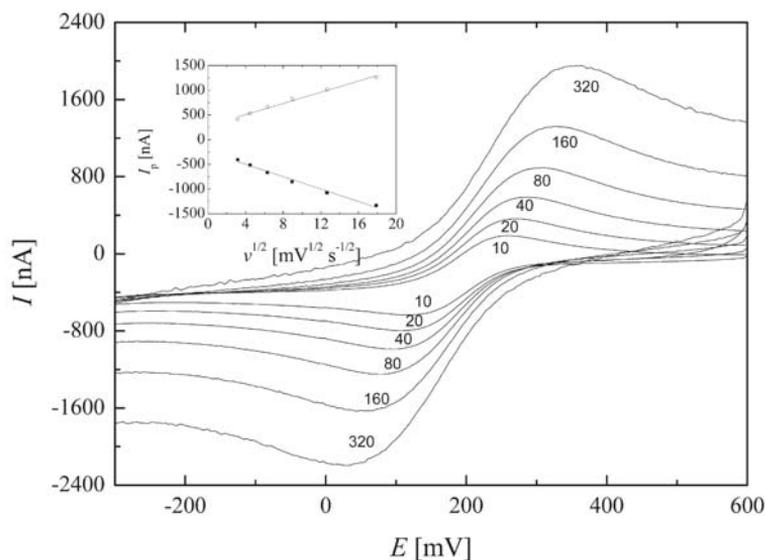
**Fig. 3** Cyclic voltammograms of  $10^{-3}$  mol L $^{-1}$  K $_3$ [Fe(CN) $_6$ ] in 0.1 M KCl at BDDFE, scan rate 10–320 mV s $^{-1}$ . Corresponding scan rates values are near the curves. Dependencies of  $I_p / v^{1/2}$  in the graph inset.
