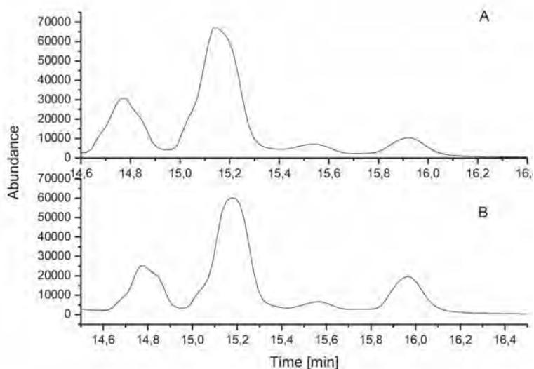
**Fig. 3** GC-MS chromatogram (A) 1% solution of butter, (B) 1% solution of butter with 5% solution of sunflower oil.
