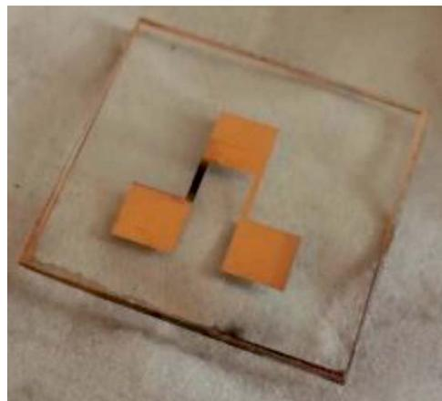
**Fig. 3** The sensing element of the gas microsenors on chip-based.
