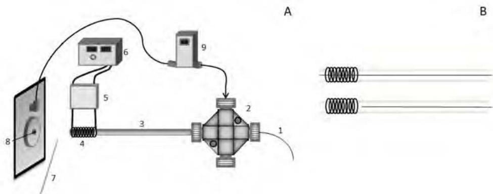
**Fig. 1** (a) Schematic view of a micro-APCI source with a tube nebulizer and (b) two different positions of fused silica capillary ending. Fused silica capillary (1), low-pressure PEEK cross (2), tube (3), resistance wire (4), ceramic terminal block (5), power supply (6), APCI needle (7), MS inlet (8), mass flow controller (9).
