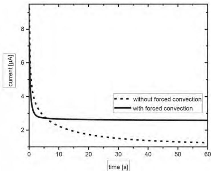
**Fig. 4** Chronoamperometric response of the substrate electrode for the oxidation of ferrocene-methanol;  $E_{\text{substrate}} = 0.45 \text{ V}$ ; quiet time: 0 s; sample time: 0.1 s; flow rate for convection: 2.1 ml/min.
