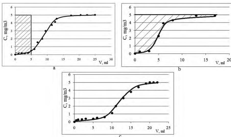
Fig. 2 Sorption curves of the studied microsystems (a)  $\text{Al}_2\text{O}_3$ , (b) MN-202, (c) CNT.
