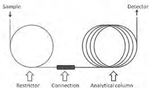
**Fig. 2** Scheme of low pressure gas chromatography (LPGC).
