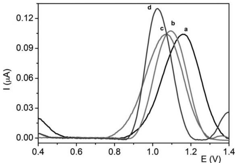
**Fig. 2** DP voltammograms of  $50 \mu\text{mol L}^{-1}$  *o*-cresol in Britton-Robinson buffer pH = 2.0 registered at BDD electrodes deposited at B/C ratio: (a) 500, (b) 1000, (c) 4000, (d) 8000 ppm.
