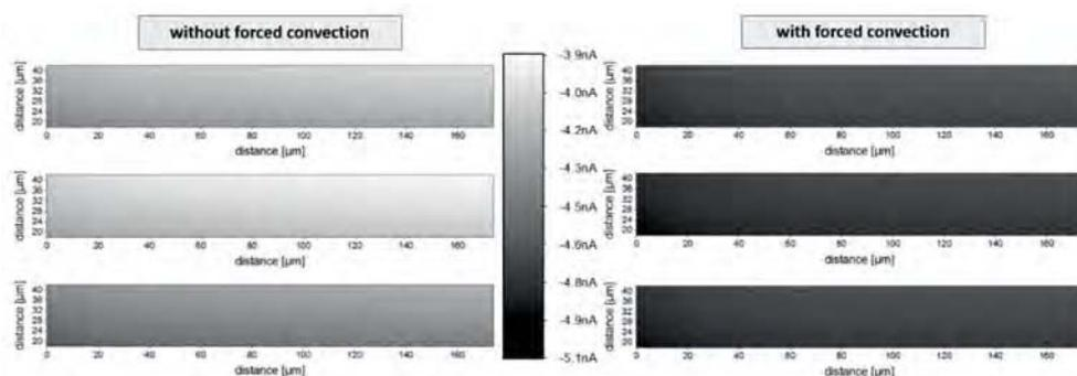
**Fig. 5** Three repetitive SECM images within the diffusion layer of the substrate electrode without and with convection in SG/TC mode.  $E_{\text{substrate}} = 0.45 \text{ V}$ ;  $E_{\text{probe}} = 0 \text{ V}$ ; scan rate:  $100 \mu\text{m/s}$ ; increment:  $6 \mu\text{m}$ ; quiet time:  $1 \text{ s}$ ; probe diameter:  $25 \mu\text{m}$ ; flow rate for convection:  $2.1 \text{ ml/min}$ .
