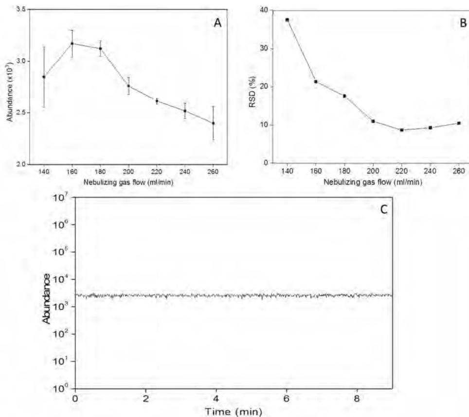
**Fig. 4** (a) Absolute signal intensity of acridine as a function of nebulizing gas flow for analyte flow rate  $1.0 \mu\text{l}/\text{min}$ , (b) corresponding *RSD* values from the same measurement, (c) stability of absolute acridine signal for gas flow rate  $220 \text{ ml}/\text{min}$ .
