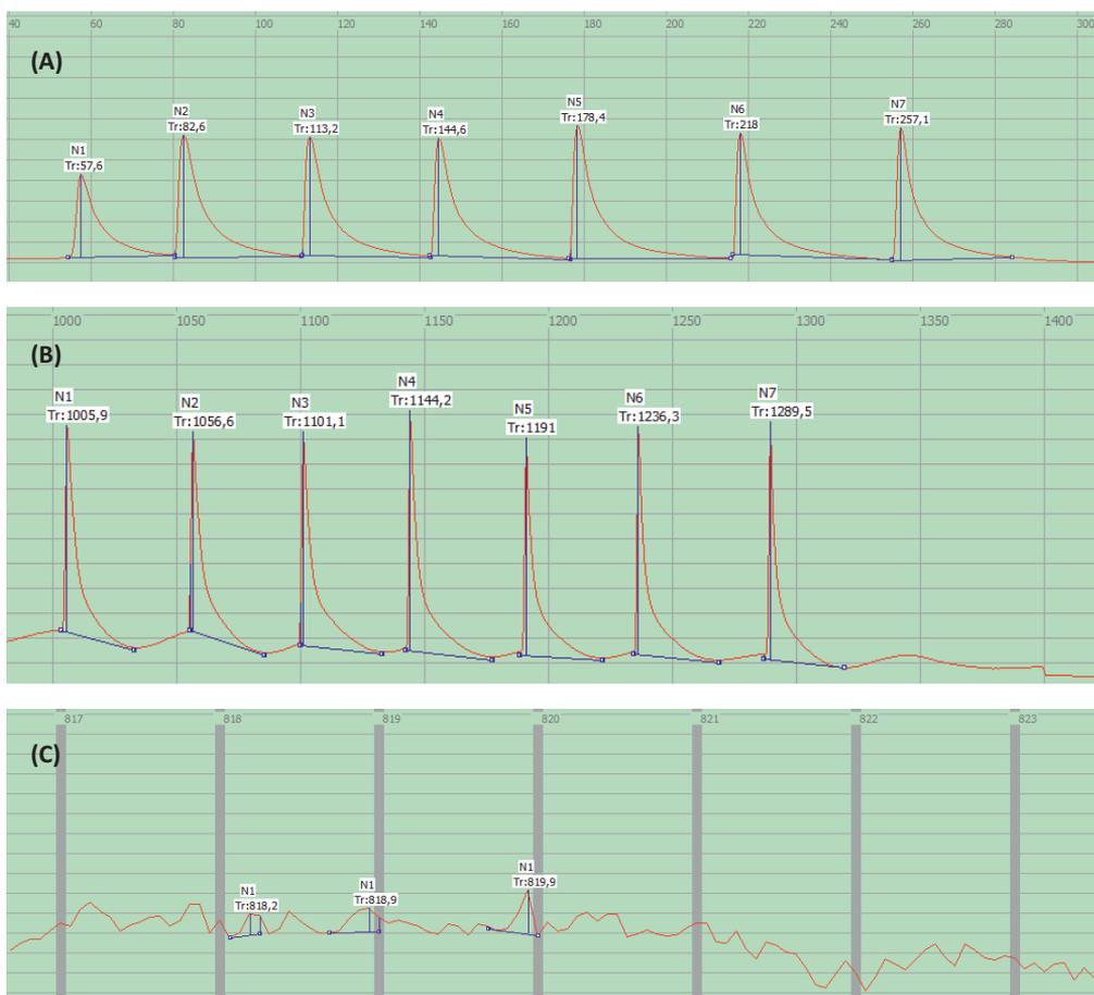
Fig. 5 (A) Chromatogram of methane. (B) Chromatogram of hydrogen. (C) Noises on the chromatogram.
