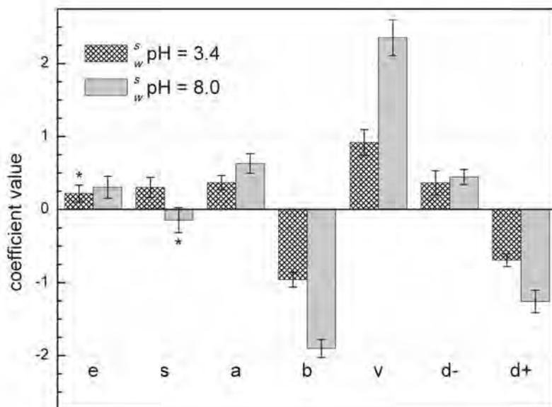
**Fig. 3** System coefficients for different  $s_w$  pH values of the eluent, provided with error bars denoting coefficient standard error and asterisks marking statistical insignificance of the coefficients.
