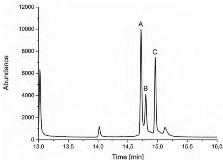
**Fig. 2** GC-MS chromatogram of separation of the standard solution of flavonol glycosides: (A) quercetin 3-O-β-D-galactoside, (B) quercetin 3-O-β-D-glucoside, (C) quercetin 3-O-α-D-arabinoside.
