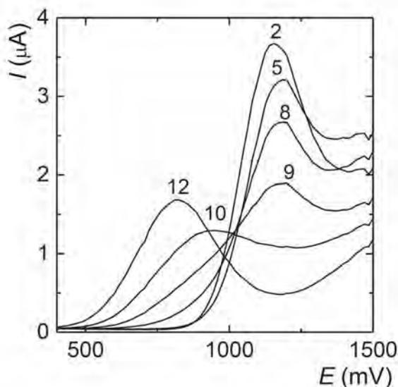
**Fig. 1** DP voltammograms of *m*-cresol ( $1 \times 10^{-4}$  mol L $^{-1}$ ) measured at boron doped diamond electrode in different pH = (2.0–12.0) of Britton-Robinson buffer indicated by the curves.
