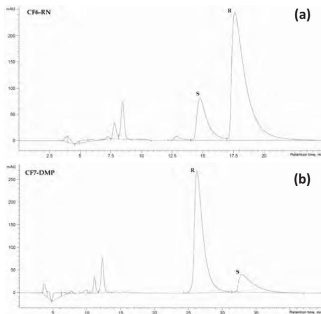
**Fig. 1** Enantioseparation of selected synthesized enantiomer on (a) CF6-RN, and (b) and CF7-DMP. Mobile phase *n*-hexane:2-propanol:trifluoroacetic acid (80:20:0.1, v/v/v); flow rate 0.8 mL min<sup>-1</sup>; detection on 250 nm.
