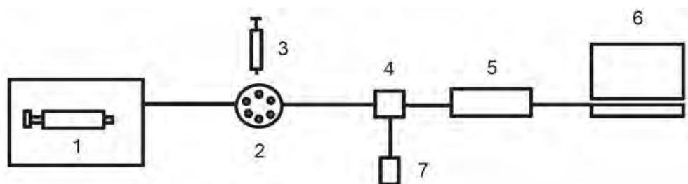
**Fig. 1** Scheme of flow injection analysis apparatus: (1) syringe pump, (2) injection valve, (3) syringe for injection of samples, (4) flow cell, (5) potentiostat, (6) computer, (7) waste.
