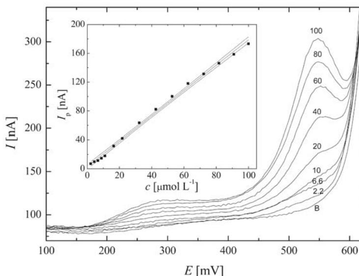
**Fig. 4** DPV curves of 0–100  $\mu\text{mol L}^{-1}$  vanillylmandelic acid at BDDFE in 0.1 M NaOH. BDDFE cathodically pretreated at  $-1000$  mV for 15 s. Corresponding vanillylmandelic acid concentrations are displayed near curves, 0.1 M NaOH blank sample (B). Inset shows linear dependency of the peak current of vanillylmandelic acid on the concentration.
