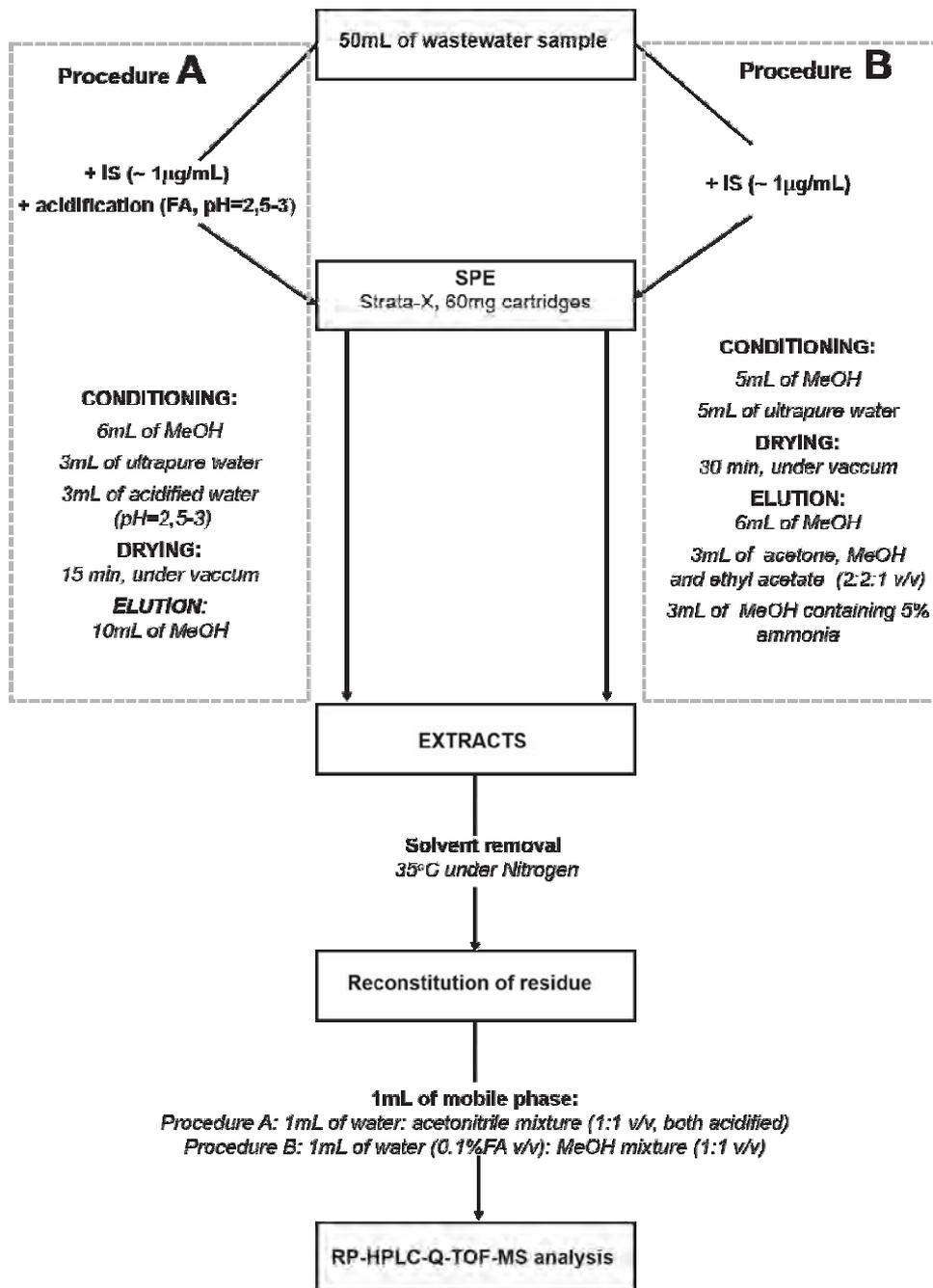
Fig. 1 Scheme of used two extraction procedures.
