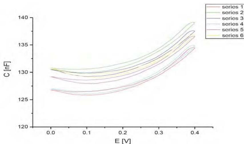
**Fig. 3** Six capacitance-potential curves recorded in 0.1 M phosphate buffer solution at pH = 7.4 as a repeatability checking of gold surface modification by using of thiols (scan rate  $50 \text{ mV s}^{-1}$ ).
