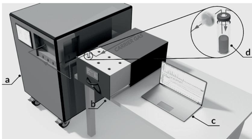
**Fig. 1** Experimental setup comprised of (a) PTR-TOFMS, (b) custom heater/incubator, (c) personal computer with data processing software, and (d) headspace vial with a syringe filter.
