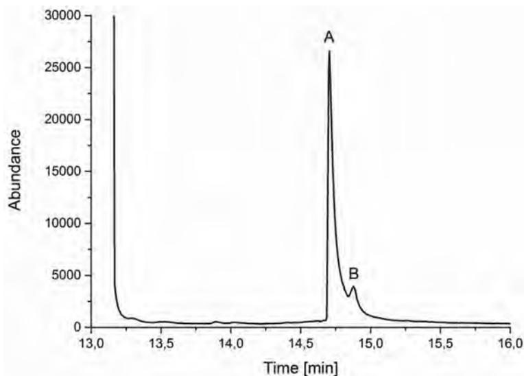
**Fig. 3** GC-MS chromatogram from separation of observed flavonol glycosides in sample 3 nutrition supplement: (A) quercetin 3-O-β-D-galactoside, (B) quercetin 3-O-β-D-glucoside.
