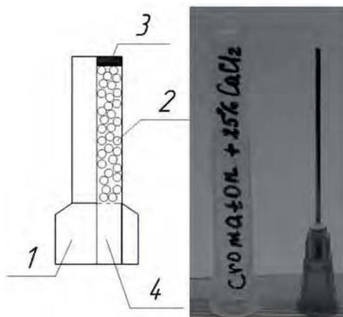
**Fig. 1** (a) The schematic diagram of micro ChDmS, and (b) photo of fabricated device (1) needle hook, (2) sorbent, (3) plug, (4) internal channel of needle.
