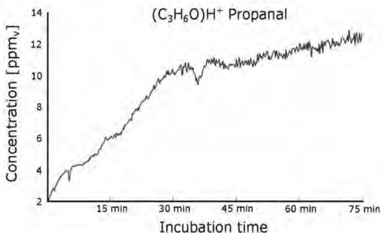
Fig. 2 Monitored concentration of propanal in olive oil fumes during incubation.
