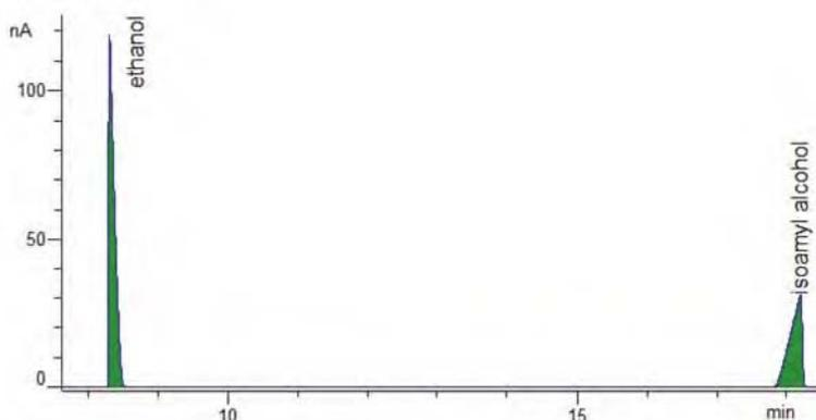
Fig. 3 Chromatogram of the prepared solution with noticeable amount of isoamyl alcohol.
