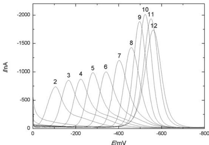
**Fig. 2** DP voltammograms of  $1 \times 10^{-3}$  mol L $^{-1}$  anthraquinone-2-sulfonate in Britton-Robinson buffer pH = 2–12 at p-AgSAE; initial potential 0 mV, final potential –1000 mV, scan rate 100 mV s $^{-1}$ , negative regeneration potential –1100 mV, positive regeneration potential +80 mV. Number of regeneration cycles 200; numbers (2–12) above the voltammograms correspond to pH of the Britton-Robinson buffer used [5].
