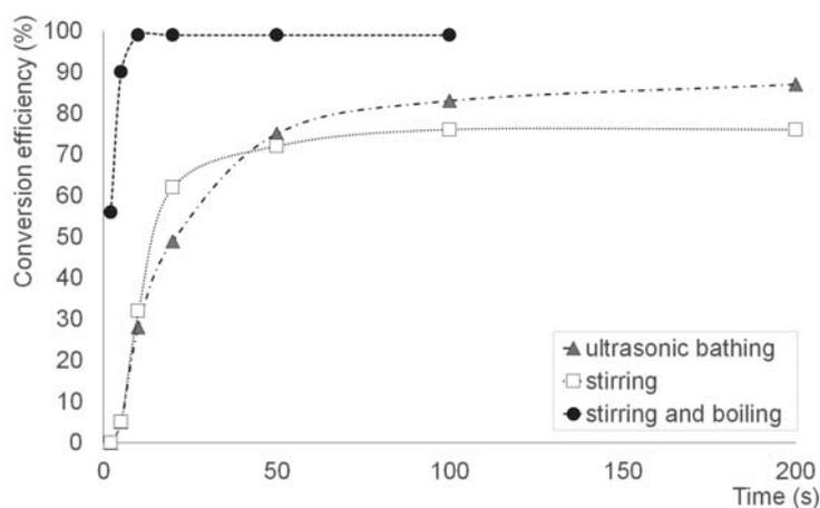
Fig. 3 Relationship between leucine conversion efficiency and time for different reaction supports.
