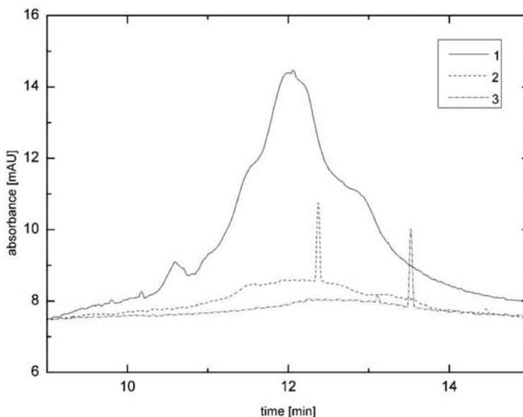
**Fig. 1** Time course of starch degradation by  $\alpha$ -amylase in offline mode. The initial concentration of starch was 0.1% w/v. Experiment was conducted in 10 mM phosphate buffer of pH = 7.0 at 37°C. Aliquots were measured after (1) 9.5 min, (2) 29.5 min, and (3) 52 min. Capillary electrophoresis conditions: 20 mM acetate buffer of pH = 5.0 with addition of 1.2 mM iodine as background electrolyte,  $U = 20$  kV.
