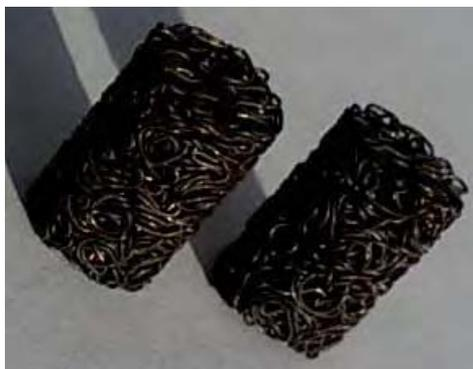
**Fig. 1** The photo of samples of metallorubber-based sorption materials.
