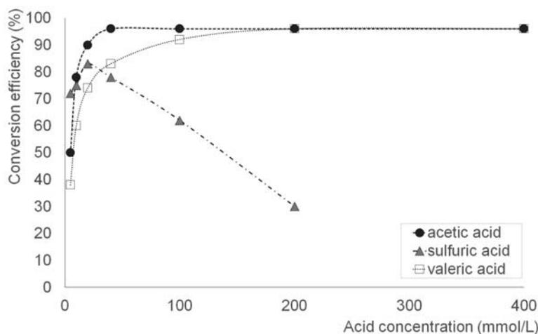
**Fig. 2** Dependence of leucine conversion efficiency on acid concentration for different acids (concentration of sodium nitrite 100 mmol/L).
