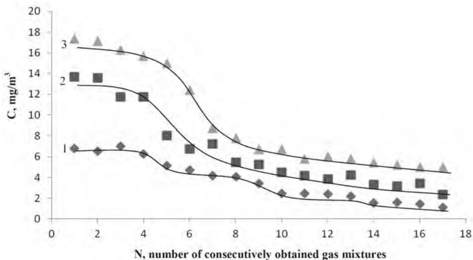
**Fig. 3** Relation between *n*-pentane concentration and the number of consecutively obtained gas mixtures with the use of ChDmS filled with carbon nanotubes: (1) desorption temperature 50 °C, (2) desorption temperature 70 °C, (3) desorption temperature 100 °C.
