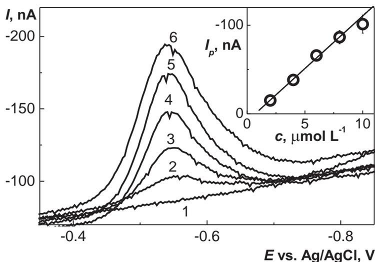
**Fig. 2** Cathodic DP voltammograms of HNN of concentration (1) 0.0, (2) 2.0, (3) 4.0, (4) 6.0, (5) 8.0, and (6) 10.0  $\mu\text{mol L}^{-1}$  obtained at GCE in one drop (20  $\mu\text{L}$ ) of BR buffer (pH = 7) and DMSO (9:1) solution after 10 min in the nitrogen atmosphere measured against silver wire pseudo-reference electrode (adjusted for Ag|AgCl in the figure). The calibration curve is shown in the inset.
