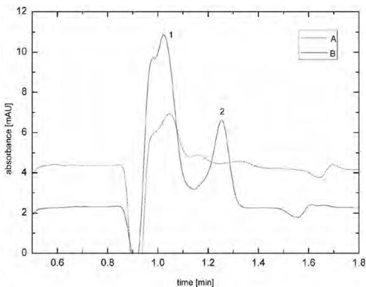
**Fig. 4** Online time course of starch degradation by  $\alpha$ -amylase. Capillary electrophoresis conditions same as in Fig. 1, measured in reversed polarity mode ( $U = -20$  kV) at  $37^\circ\text{C}$ . Different incubation times: (A) 10 min, (B) 0.5 min. Peaks: (1) amylopectin, (2) amylose.
