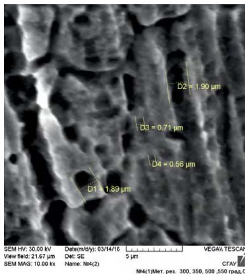
**Fig. 2** The SEM image of surface of metallorubber treated with hydrochloric acid and oxidized at 700 °C.
