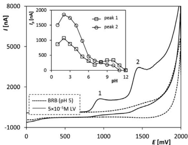
**Fig. 2** Cyclic voltammogram of leucovorin obtained on BDDE. Method: Britton-Robinson buffer pH = 5.0,  $E_{in} = E_{fin} = 0$  mV,  $E_{switch} = +2000$  mV,  $v = 100$  mV s<sup>-1</sup>,  $c(\text{leucovorin}) = 5 \times 10^{-5}$  mol L<sup>-1</sup>. Inset: dependences of  $I_p$  on pH (0.05 mol L<sup>-1</sup> H<sub>2</sub>SO<sub>4</sub> (pH = 1), Britton-Robinson buffer pH = (2–12)).
