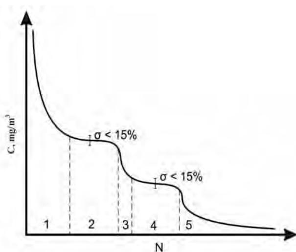
**Fig. 5** The relation between the number of consecutively obtained mixtures and their concentration: (1) ramp-up time, (2, 4) constant concentration site, (3) period of redistribution of the target component in the system, (5) system exhaustion period.
