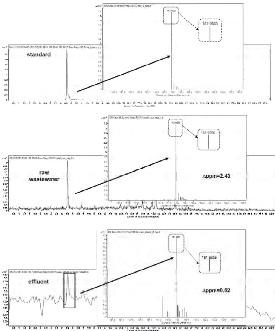
**Fig. 3** Obtained LC-MS/MS chromatograms of acesulfame-K.
