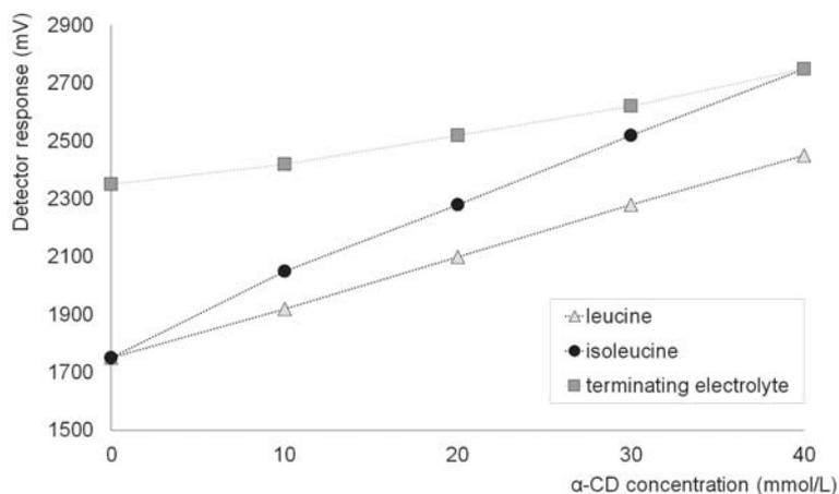
Fig. 5 Dependence of conductivity detector response on  $\alpha$ -cyclodextrine concentration in leading electrolyte (pH = 3.4).
