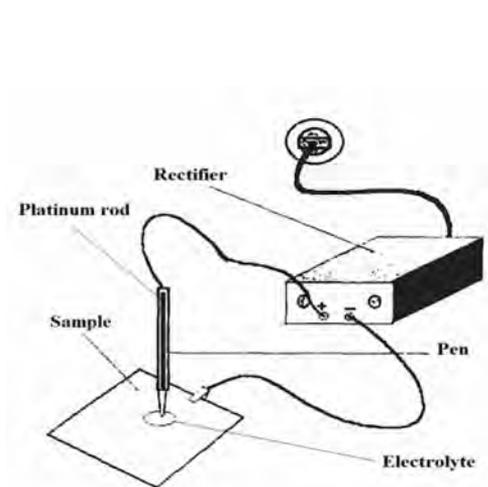
**Fig. 1** The schematic circuit of electrolytic polishing
