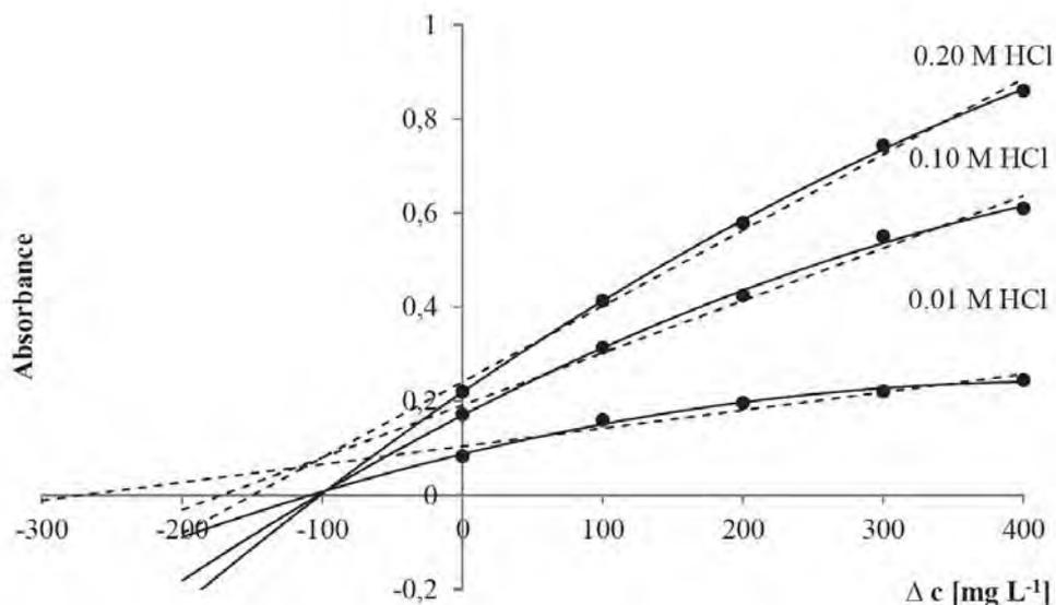
**Fig. 2** Set of calibration curves created using a linear (dotted line) and polynomial (continuous line) plot obtained for the sample of 100 mg L<sup>-1</sup> paracetamol
