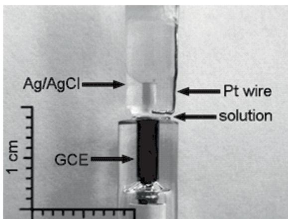
**Fig. 1** Microcell for anodic voltammetry with GCE, Ag|AgCl reference electrode and platinum wire auxiliary electrode with 20  $\mu$ L sample.
