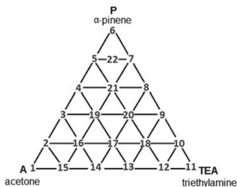
**Fig. 2** A ternary plot illustrating the composition of the tested mixtures.
