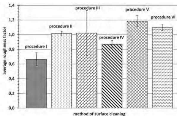
Fig. 2 Purity of electrodes surface according to used procedures of cleaning (from Table 1).
