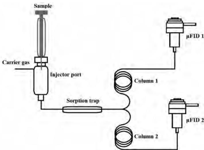
Fig. 1 Scheme of the electronic nose based on ultra-fast gas chromatography.
