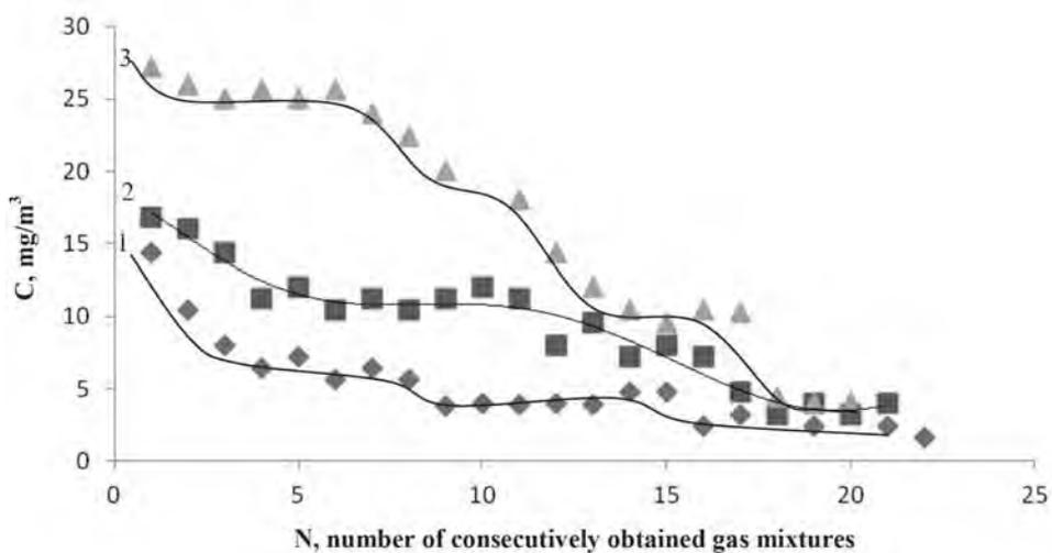
**Fig. 4** Relation between *n*-pentane concentration and the number of consecutively obtained gas mixtures with the use of ChDmS filled with  $\text{Al}_2\text{O}_3$ : (1) desorption temperature 50 °C, (2) desorption temperature 70 °C, (3) desorption temperature 100 °C.
