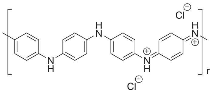
**Fig. 1** Chemical structure of partly protonated polyaniline – emeraldine salt.
