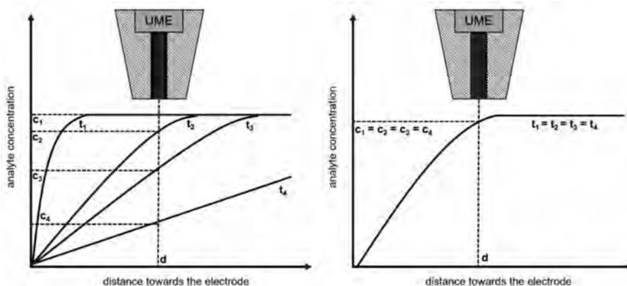
Fig. 2 Comparison of the conditions at the UME during SECM experiments in SG/TC mode without and with forced convection applied to the system.
