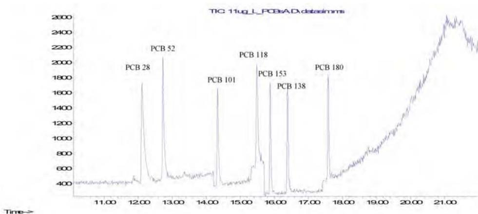
**Fig. 1** Chromatogram of standard solutions of PCBs.
