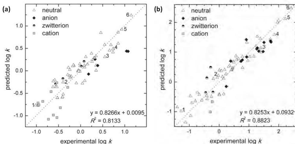
**Fig. 2** Plot of experimental vs. predicted  $\log k$  for different  $s_{\text{w}}\text{pH}$  values of the mobile phases: (a)  $s_{\text{w}}\text{pH}$  value of 3.4, (b)  $s_{\text{w}}\text{pH}$  value of 8.0 (solutes are considered to be ions if at least 10% dissociated), the dotted line denotes equal  $\log k$  values. Solutes: (1) acetone, (2) benzene, (3) naphthalene, (4) biphenyl, (5) anthracene, (6) pyrene.
