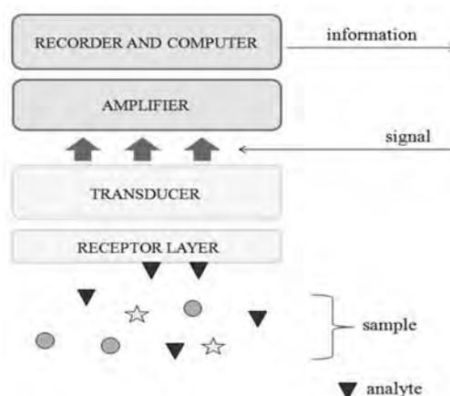
**Fig. 1** Scheme of chemical sensor according to IUPAC definition [2].
