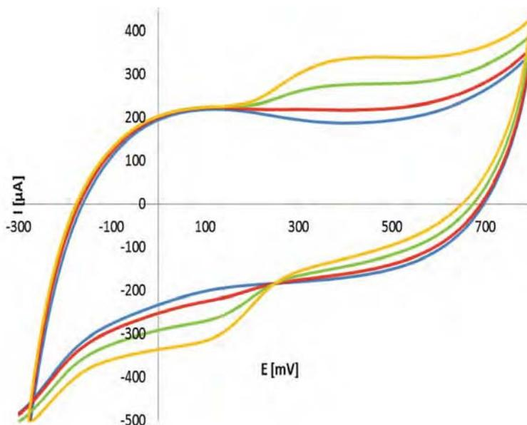
**Fig. 2** Exemplary voltammograms recorded for the best nanocomposite based on Nafion/TiO<sub>2</sub>/AuNP/buffer/CMK (30.1% / 22.8% / 9.5% / 37.6%) at scan rate of 62.5 mV s<sup>-1</sup>.
