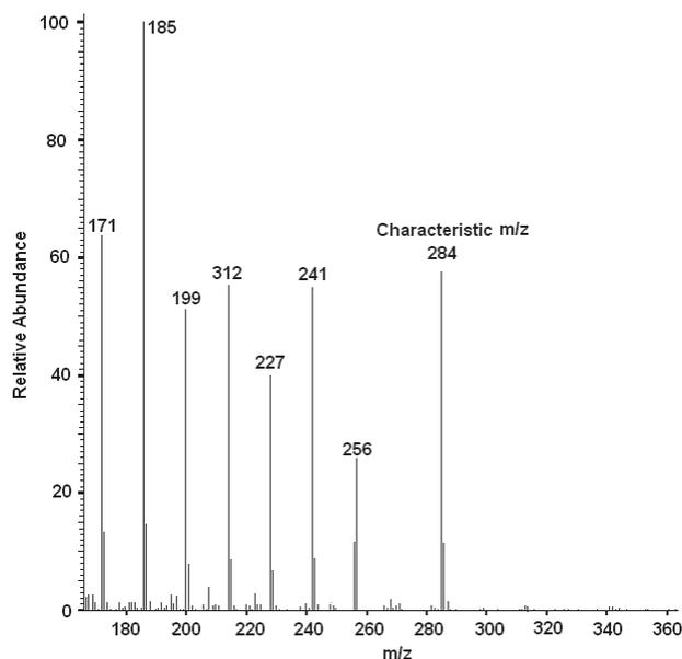
Fig. 4 Selection of the characteristic ion for stearin with mass spectra.
