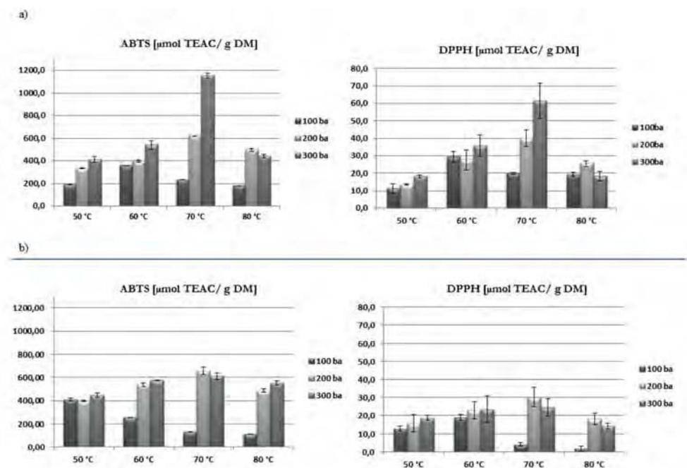
**Fig. 3** Antioxidant potential of *Medicago sativa* leaves extracts obtained with using different temperature and pressure conditions using SC-CO<sub>2</sub> with (a) 20%, and (b) 15% (v/v) ethanol as a modifier.
