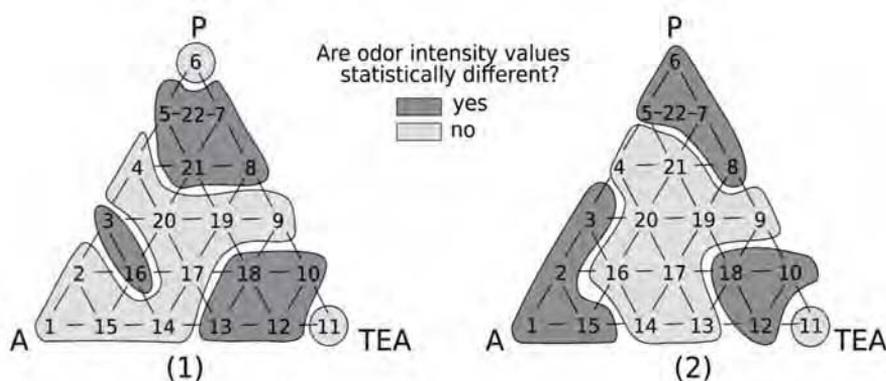
**Fig. 4** Ternary plots of gas mixtures odor intensity statistical differences: (1) determined by the sensory analysis, (2) modeled using the e-nose, compared to the values calculated using the Zwaardemaker model. Abbreviations: (P)  $\alpha$ -pinene, (A) acetone, (TEA) triethylamine.
