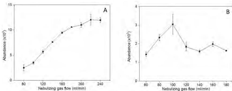
**Fig. 3** Absolute signals of acridine as a function of nebulizing gas flow rate for (a) quartz tube and (b) corundum tube.
