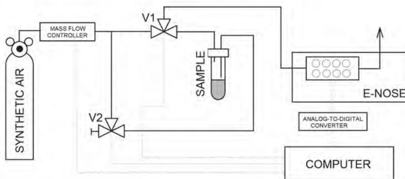
Fig. 3 Electronic-nose measurement system.
