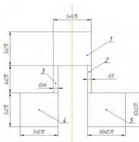
**Fig. 2** The schematic circuit of gas microsenors on chip-based: (1, 4, 5) pressure contacts, (2) microsenors with a catalytic layer of platinum, (3) microsenors without catalytic layer of platinum.
