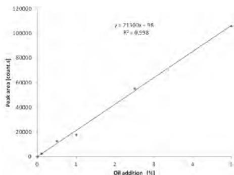
**Fig. 4** Calibration curve of the addition of sunflower oil to butter with a range of concentration from 0.1% to 5% by LPGC.
