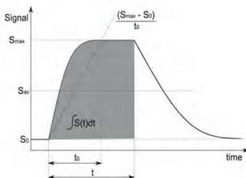
**Fig. 1** Signal parameters used for data analysis:  $S_{\max}$  is maximum signal value,  $S_{\text{av}}$  is average signal value,  $\int S(t)dt$  is integral of sensor signal,  $(S_{\max} - S_0)/t_0$  is difference quotient of signal.
