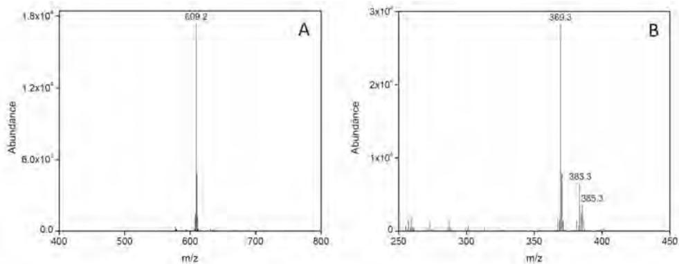
**Fig. 5** Mass spectra of (a) reserpine, and (b) cholesterol obtained with micro-APCI source with tube nebulizer.
