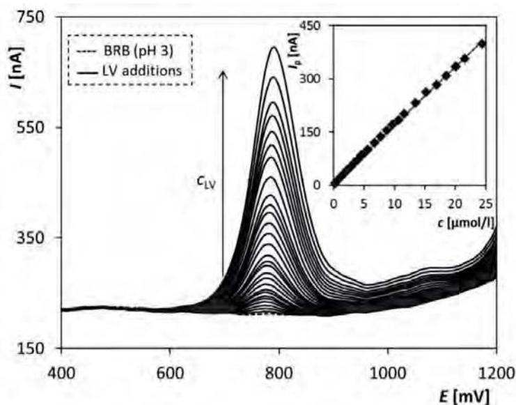
**Fig. 3** DP voltammograms of leucovorin obtained on BDDE in dependence on concentration. Method: DPV, Britton-Robinson buffer pH = 3,  $E_{in} = 0$  mV,  $E_{fin} = 1200$  mV,  $v = 40$  mV s<sup>-1</sup>, pulse height = 50 mV, pulse width = 20 ms,  $c(\text{leucovorin}) = 2.99 \times 10^{-7}$ – $2.45 \times 10^{-5}$  mol L<sup>-1</sup>. Inset: dependence of  $I_p$  on  $c(\text{leucovorin})$  for the peak 1.
