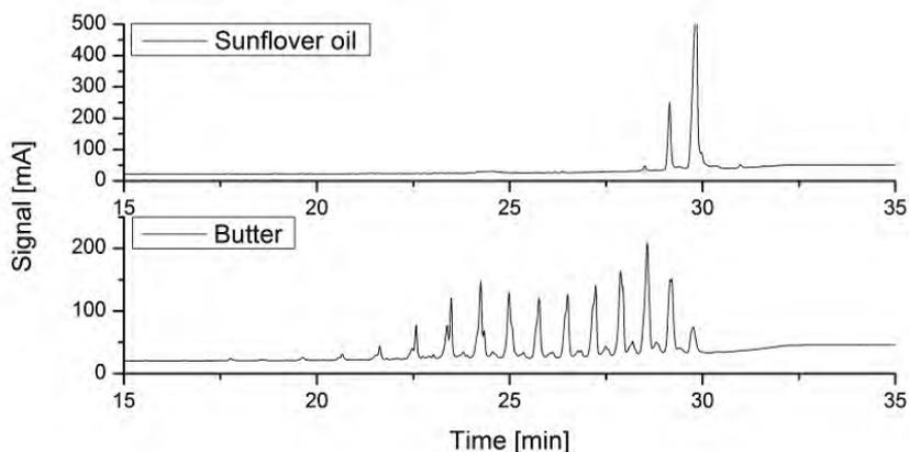
Fig. 1 Chromatogram of butter and sunflower oil using GC-FID method.
