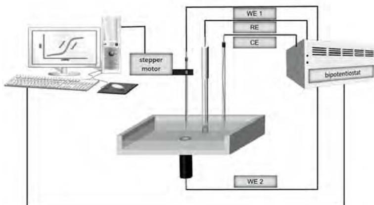
**Fig. 1** Schematic setup of the SECM. The probe, which acts as working electrode 1 (WE 1), is scanned across a surface (WE 2) via stepper motors. The electrochemical cell is completed by a reference electrode (RE) and a counter electrode (CE). The measurements are performed with a bipotentiostat controlled by a computer.
