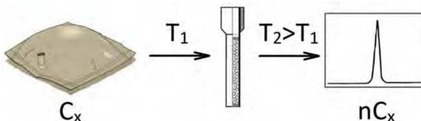
**Fig. 1** Scheme of concentrating: ( $T_1$ ) temperature of concentrating process, ( $T_2$ ) temperature of desorption, ( $C_x$ ) – analyte concentration in model gas mixture, ( $nC_x$ ) analyte concentration after concentrating.
