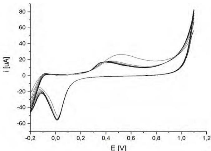
**Fig. 3** Cyclic voltammogram obtained during electrochemical cleaning of gold electrodes in potassium hydroxide solution (scan rate  $100 \text{ mV s}^{-1}$ ).
