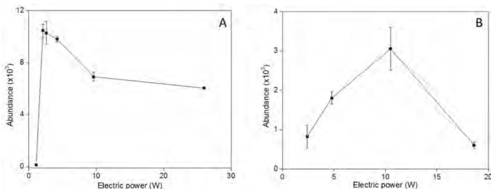
**Fig. 2** Absolute signals of acridine as a function of electric power, which was applied to the resistance wire of the (a) quartz tube and (b) corundum tube.
