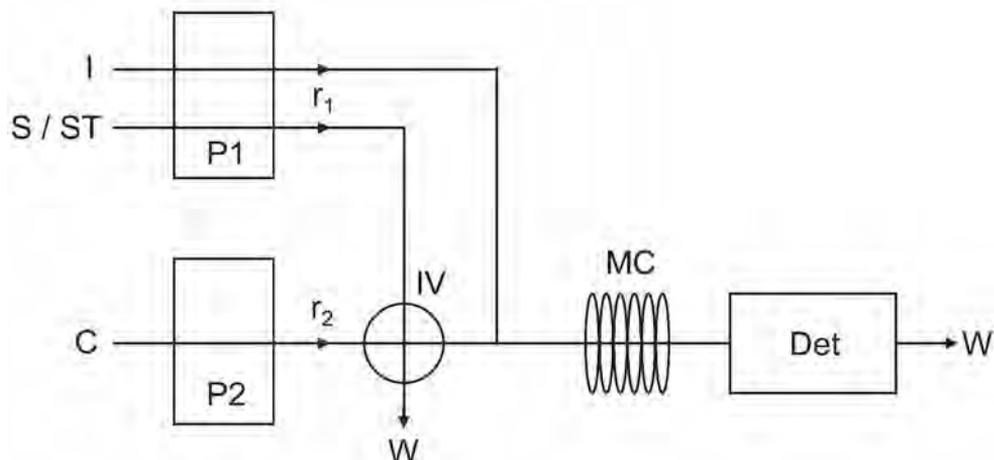
**Fig. 1** Scheme of the flow-injection system: C – carrier, ST – standard, S – sample, I – indicator, P1 and P2 – peristaltic pumps,  $r_1$ ,  $r_2$  – flow rates, IV – injection valve, MC – mixing coil, W – waste, Det – detector.
