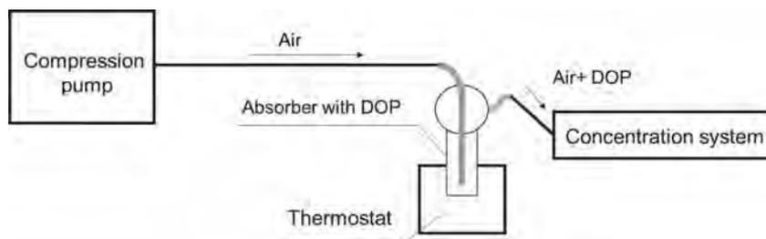
**Fig. 3** The schematic diagram of experimental device for concentration dioctylphthalate from model vapor-gas mixture.
