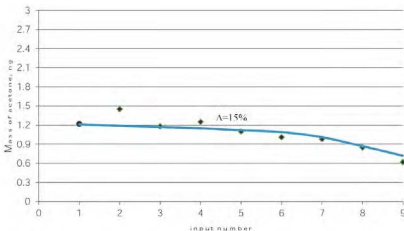
**Fig. 2** Acetone concentration in dependence on ChDmS filled Cromaton N-AW-DMCS + 25% CaCl<sub>2</sub> sorbent usage period under conditions of discrete dosing.
