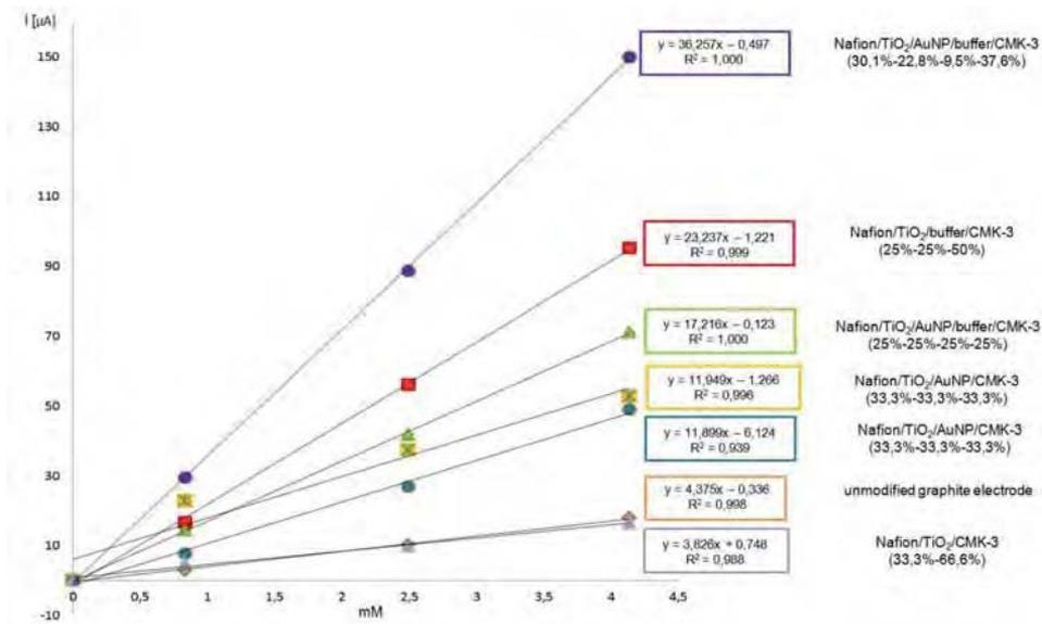
**Fig. 1** Obtained calibration curves towards Fe(II)/Fe(III) redox probe for various matrix including components mixed in different volumetric ratio.
