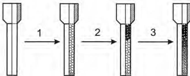
**Fig. 1** Stages of chromatodesorption system production: (1) filling with a sorbent, (2) saturation with a target component, (3) preparation procedure.
