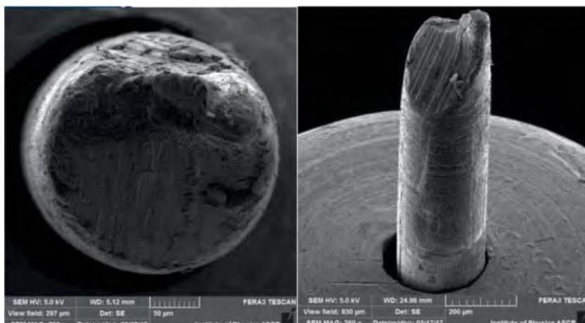
**Fig. 2** SEM image of used boron doped diamond film electrode. Boron doped diamond film deposited on titanium wire by micro-wave assisted plasma CVD.
