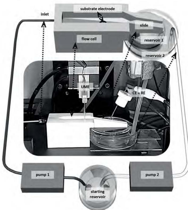
Fig. 3 Experimental setup. Developed electrochemical flow cell integrated into the SECM instrument.
