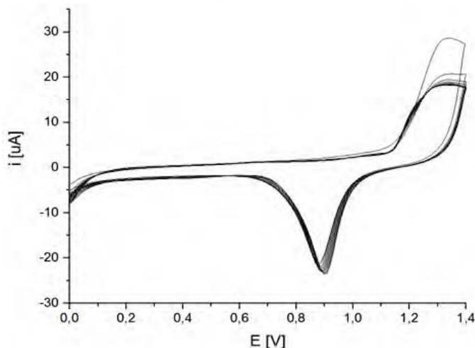
**Fig. 1** Cyclic voltammogram obtained during electrochemical cleaning of gold electrodes in sulfuric acid solution (scan rate  $100 \text{ mV s}^{-1}$ ).
