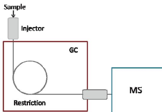
Fig. 1 Schematic diagram of GC-MS system without chromatographic separation.
