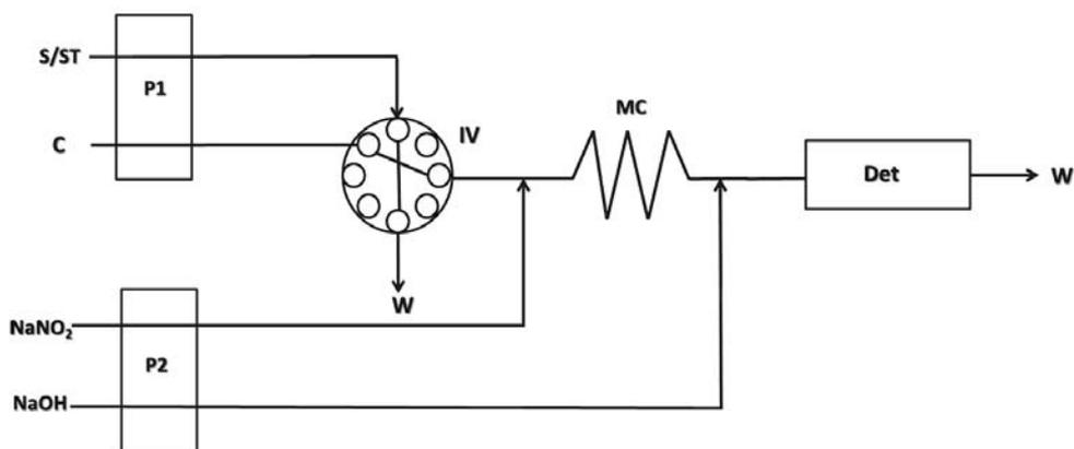
**Fig. 1** Scheme of the employed flow-injection system: (C) carrier stream, (ST) standard solution, (S) sample solution, (P1, P2) peristaltic pumps, (IV) injection valve, (MC) mixing coil, (W) waste, (Det) detector.
