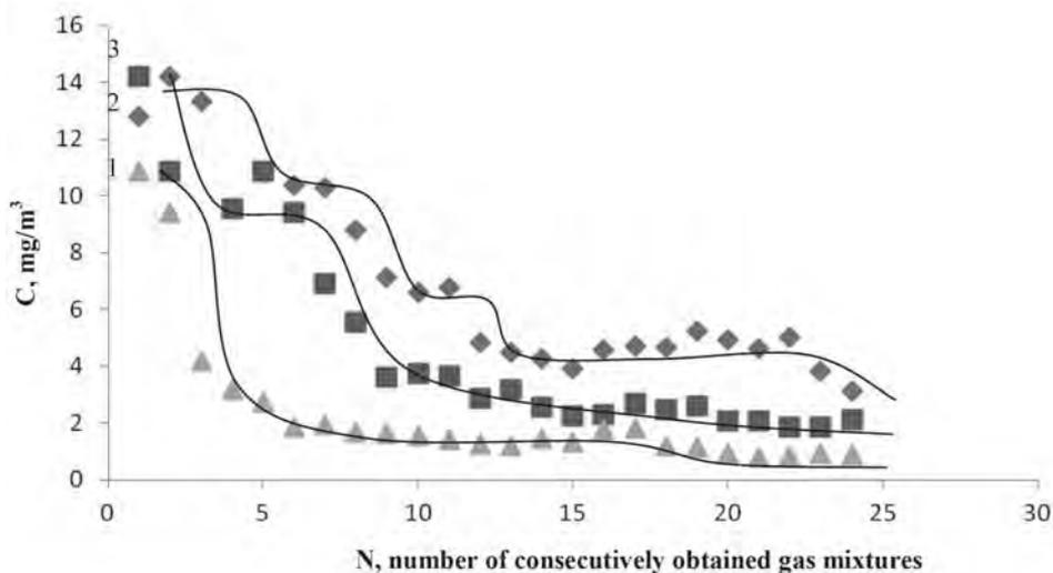
**Fig. 2** Relation between *n*-pentane concentration and the number of consecutively obtained gas mixtures with the use of ChDmS filled with fibreglass with 15% PMS-1000: (1) desorption temperature 50 °C, (2) desorption temperature 70 °C, (3) desorption temperature 100 °C.
