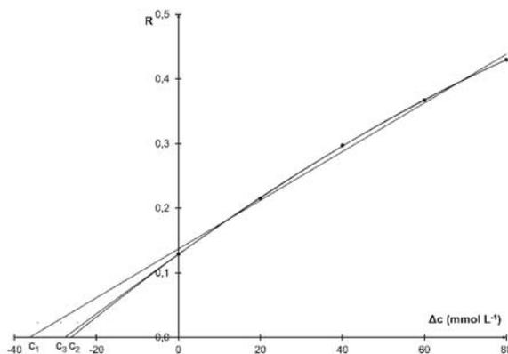
**Fig. 2** Calibration curves obtained in the standard addition method for the synthetic sample;  $c_1$ ,  $c_2$ ,  $c_3$  are analytical results calculated by extrapolation of linear, polynomial of degree 2, and polynomial of degree 3 functions, respectively.
