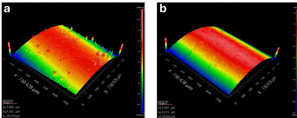
**Fig.2** Profilometry image of polymer layers on brass cartridges: (a) poly(neutral red), (b) poly(toluidine blue).
