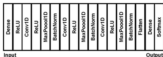
**Fig. 2** Architecture of 1D Convolutional Neural Network
