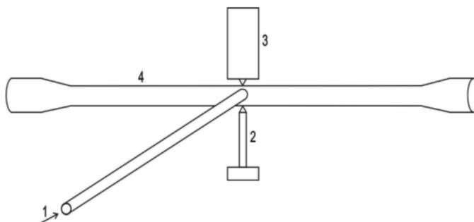
**Fig. 1** Scheme of atmospheric pressure glow discharge atomizer: (1) inlet arm, (2) tungsten anode, (3) brass cathode with tungsten tip, (4) optical arm.
