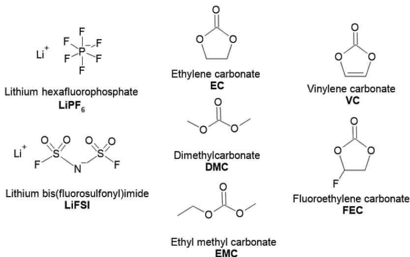
**Fig. 1** The chemical formulas of the single components in the electrolyte. On the left the conductive salt: lithium hexafluorophosphate (LiPF<sub>6</sub>) and lithium bis(fluorosulfonyl)imide (LiFSI). In the middle a variation of electrolyte solvents: ethylene carbonate (EC), ethyl methyl carbonate (EMC), dimethyl carbonate (DMC). On the right side the electrolyte additives: vinylene carbonate (VC) and fluoroethylene carbonate (FEC).
