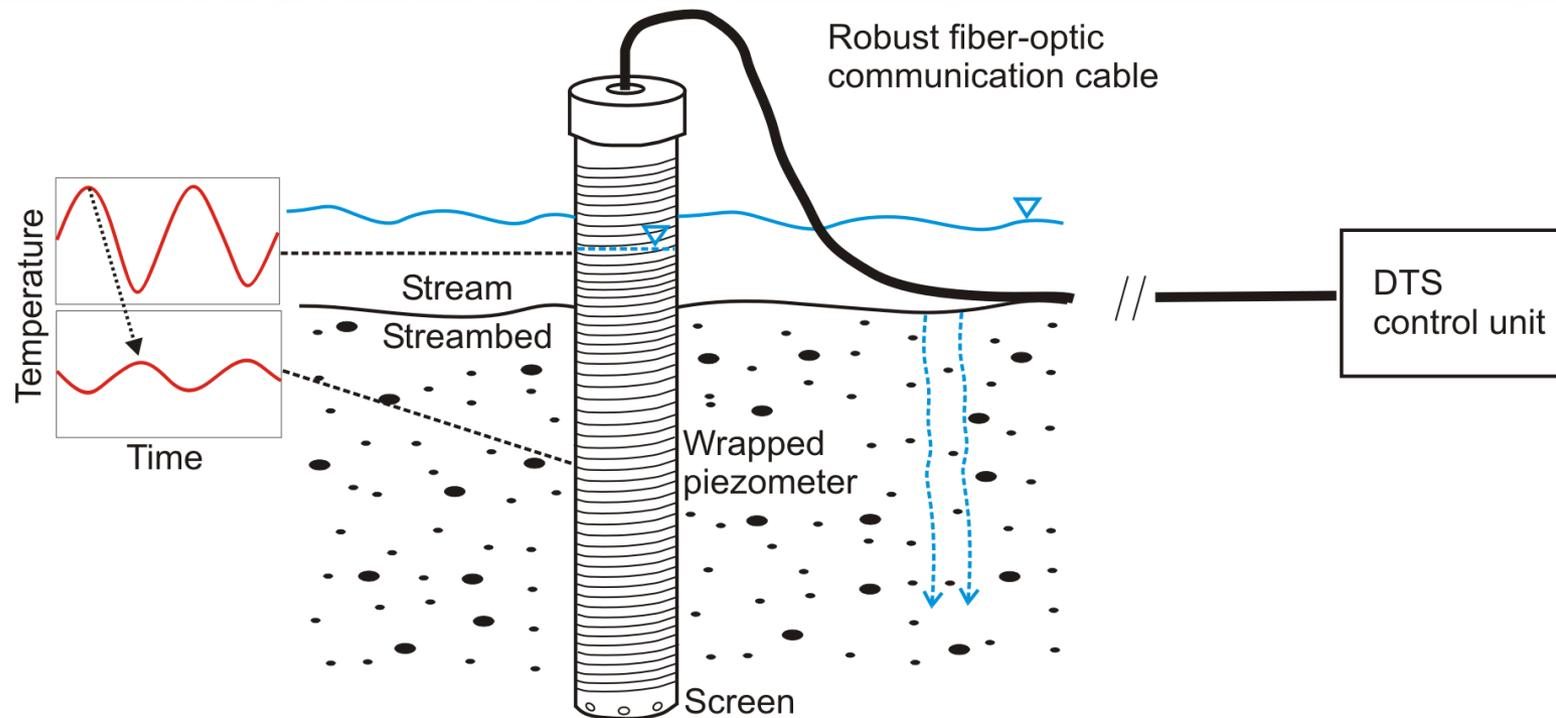
Wrapping around a 2" piezometer-tube (PVC):
