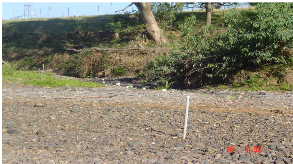
Figure 2. Location of in-stream piezometers used to delineate upwelling/downwelling process at the Ballantines transect. The picture was taken during a dry spell of 2009.
