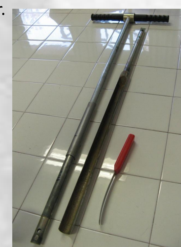
Fig. 2 - Eijelkamp Agrisearch auger equipment.
