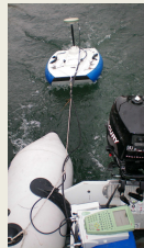
Fig.4. Bathymetry data collection using depth sounder Sontek/YSI RiverSurveyor M9 and GPS differential 1200 Leica.
