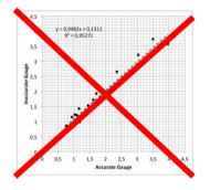
It cannot be solved with linear regression. One must solve it using data assimilation techniques such as Bayesian combination and or Filters (KF, EnKF, Particle Filter, etc.)
