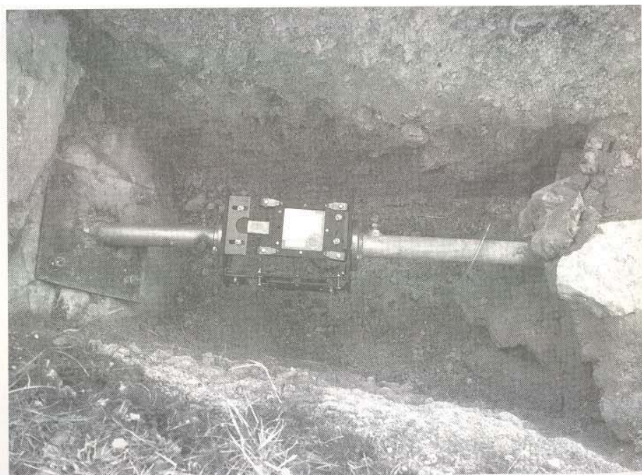
Photo 2 A Crack Gauge TM 71 installed in the Colfiorito Basin (Photo by V. Vilimek)
