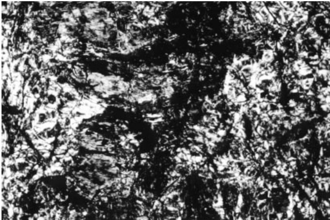
Fig. 16. Serpentinized peridotite, GU. Vraník village, SE of Leděčko. Note the relics of pyroxene (top right) in completely serpentinized matrix; polarized light; magn. 37x.
