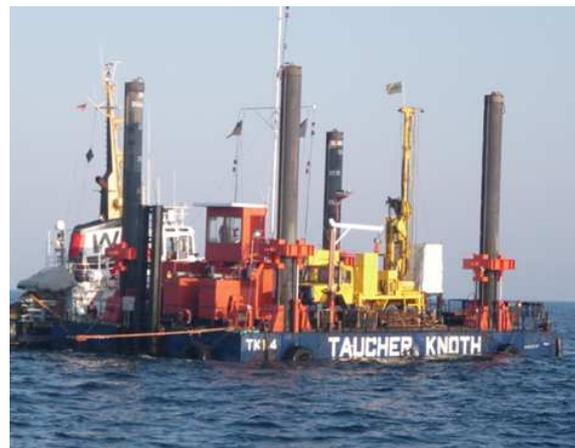
Figure 4. Platform with onshore CPT equipment
