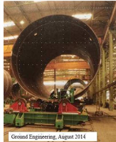
A very topical application of steel pipe piles is in the offshore wind industry, where extremely large diameter ‘monopiles’ have provided the primary foundation choice for developments in European coastal waters of the North Sea.
