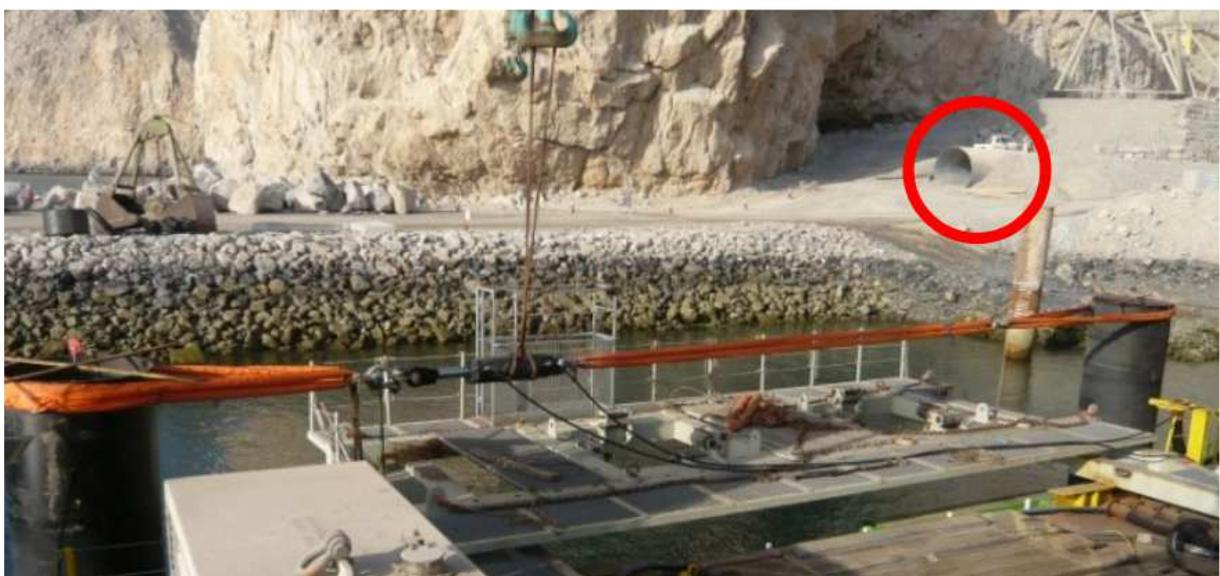
Figure 5. (a) Horizontal load set-up (testing two fender piles simultaneously)
