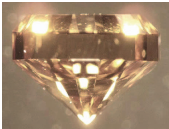
FIGURE 2 Modified, brilliant-cut, single-crystal diamond grown by CVD. The crystal is 2.45 mm high and was grown in one day. The top 0.5 mm (table) of the crystal is a yellow Type Ib HPHT substrate; thus the yellow tint is due to internal reflection (the CVD diamond is transparent and colorless) (Yan et al. 2004).
