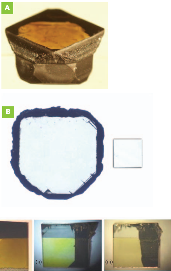
FIGURE 3 A. Photograph of a typical, three-dimensional, as-grown CVD crystal sitting atop a type 1b substrate. The CVD layer is 1.2 mm thick and was grown in 12 hours. The yellow color is due to the substrate. B. Left: 5 × 5 × 0.5 mm diamond plate grown in about 5 hours by CVD. Right: plate produced by De Beers. C. Color changes after HPHT annealing: (i) brown, as-grown CVD layer deposited on yellow type 1b HPHT seed; (ii) annealed at 1900°C and 6.5 GPa for 1 hour—CVD layer turned blue; (iii) annealed at 2200°C and 7.0 GPa for 10 hours—CVD layer turned colorless while the substrate became light yellow (from Charles et al. 2004).
