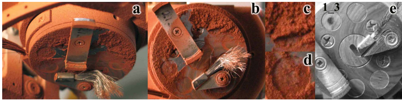
Figure 4. The RAT after abrading the UT97–20B. (a and b) Two different positions of the RAT, (c) the RAT 1_3 magnet, and (d) the RAT2 magnet. These two magnets did not collect any piles of dust that are believed to be held by magnetism. It appears that the fine reddish dust on the RAT is mainly held by electrostatic forces. (e) The Ouro Preto used as hematite analog by Goetz et al. [2008]. Here dust is clearly collected on RM1_3.
