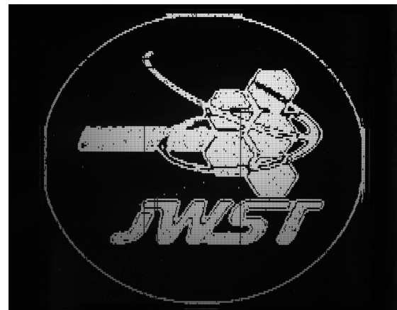
Figure 15. A 2-dimensional addressing pattern in a MSA.
