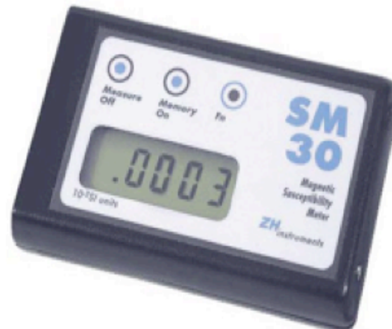
Figure 2: Magnetic susceptibility is measured by using sensitive magnetic susceptibility meter SM30, placed against the forehead. Sensitivity is 1e-7 SI units. Meter consists of 50 mm pickup coil, placed parallel with the bottom part of the cover (not seen in this figure). Weight 0.018 kg, Operating frequency: 8 kHz, Operating range -20C to 50C, Battery: 2 lithium 3V type CR2430. The meter contains an oscillator with the pickup coil. The frequency of the oscillator depends on the distance of the meter from the sample. The change in frequency is proportional to the amount of susceptibility of the rock.
