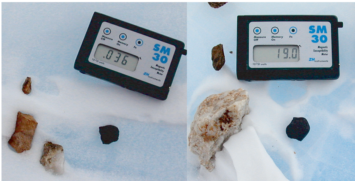
FIG. 5. Magnetic susceptibility ( K ) measurement using the SM30 on an Antarctic blue ice field during the XX Programma Nazionale di Ricerche in Antartide expedition, showing the different output between a terrestrial schist (left) and a meteorite (right). After Folco et al. (2006).
