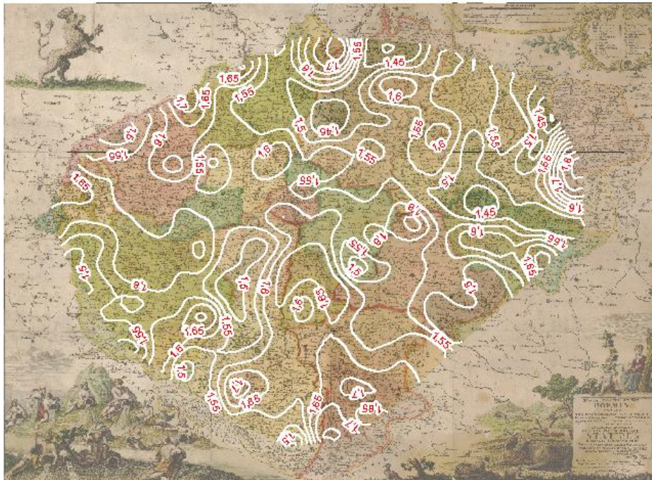
Figure 4: Scale isolines of the longitudes of Vogt's map generated with the step 0.05.
