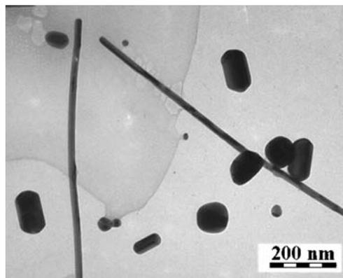
**FIGURE 1** TEM image of parent (as-prepared) citrate-reduced Ag hydrosol containing Ag nanowires
