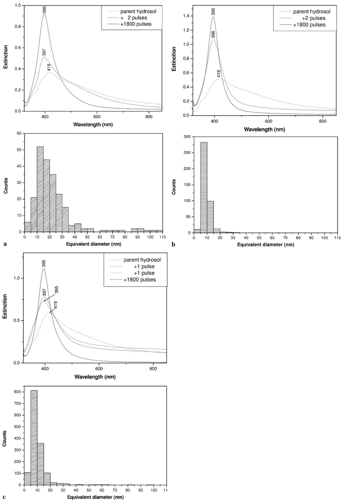
**FIGURE 2** SP extinction spectra of Ag hydrosols after varying numbers of fragmenting pulses of **a** 1064 nm, **b** 532 nm and **c** 355 nm wavelengths. *Dot-dotted curve* – original hydrosol, *dashed line* – after first fragmentation pulse, *dashed and dotted line* – after two fragmentation pulses, *straight line* – after 1800 pulses (3 min). Nanoparticle size distribution histograms of Ag hydrosols at the final stage of fragmentation at each of the above wavelengths are also presented
