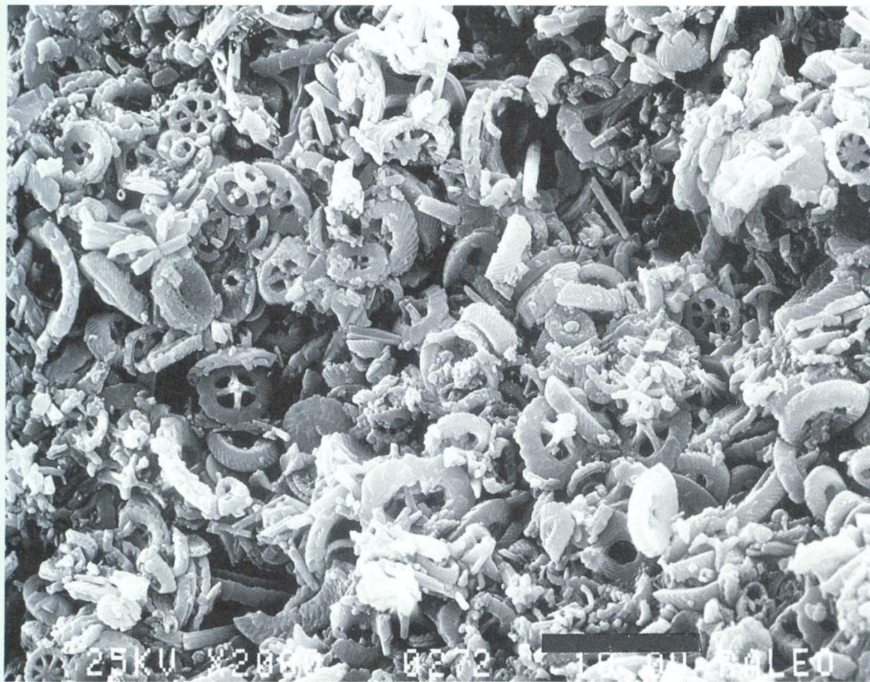
Figure 13— A. (left) Scanning electron microscope (SEM) photograph of epicon-tinental shelf chalk from Smokey Hill Shale Member of the Niobrara Formation. Sample shows well preserved, varied assemblage of coccoliths and rhabdoliths and porosity in the 35 to 40% range; scale bar is 10 \mu\text{m} . B. (below) SEM photograph of typical Tertiary deep-sea chalk from the Hatton-Rockall Basin. Note minor corrosion of coccolith margins. DSDP Leg 12, Site 116 at 462-m burial depth. Scale bar is 4.5 \mu\text{m} .
