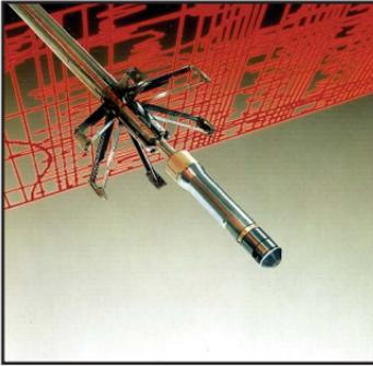
This photograph shows a six arm dipmeter tool that measures six radii or three diameters of the wellbore for accurate hole volumes. Copyright © Halliburton Energy Services.
