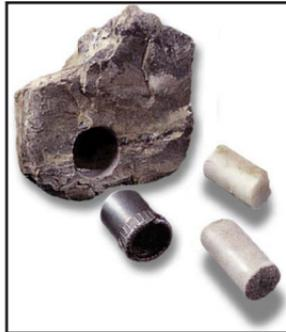
The photographs shown above are of a rotary sidewall coring tool and the subsequent cores that have been taken. Notice the miniature drill bit used to drill the core. Copyright © Halliburton Energy Services.
