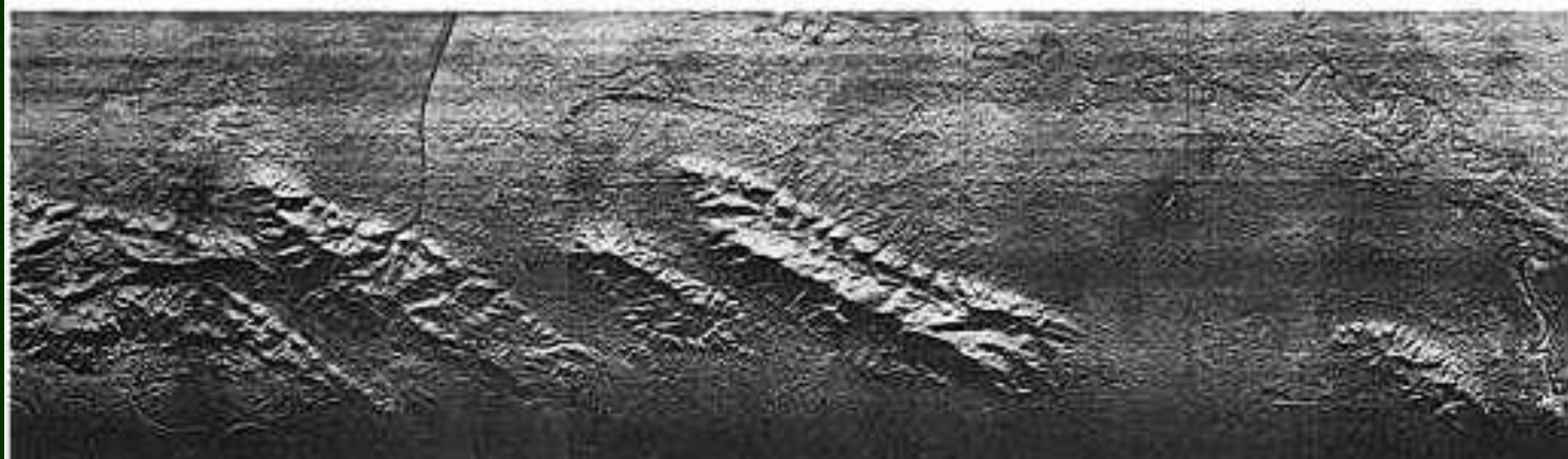
FIGURE 19.13 A side-scan radar image from the Darien Basin in eastern Panama showing an array of en echelon anticlines whose formation has arched up the land surface, creating a set of ridges. The field of view is about 50 km. Note that the geometry of these structures indicates left-lateral shear.
