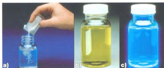
FIGURE 20.4 Detection of indicator bacteria with Colilert. (a) Addition of salts and enzyme substrates to water sample; (b) yellow color indicating the presence of coliform bacteria; (c) fluorescence under long-wave ultraviolet light indicating the presence of E. coli . Photographs courtesy of IDEXX, Westbrook, ME.
