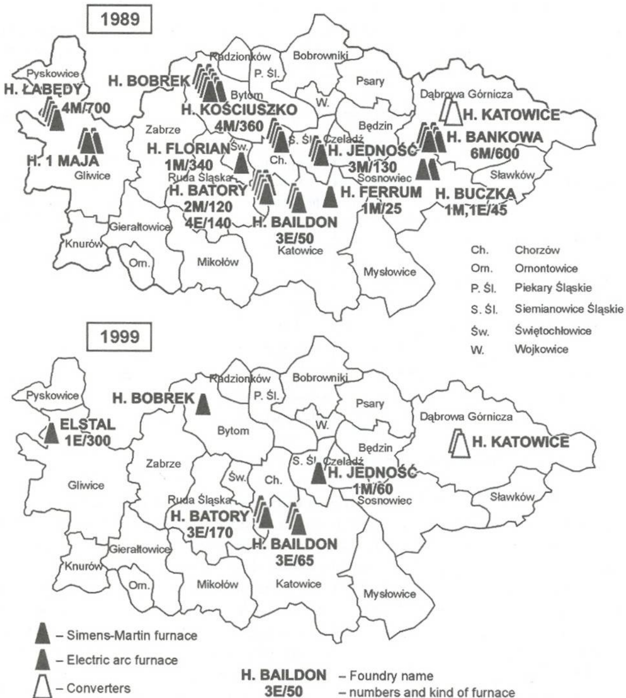
Fig. 3 Distribution and characteristics of steel plants throughout the steelworks of the GOP district in 1989 and 1999
