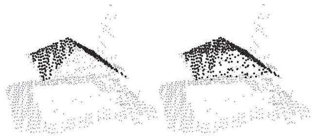
Fig. 4 Points that are excluded from the calculation in the case of fitting a gable roof model (left) and a hip roof model (right) to a hip roof type. In the case of a gable roof model, the points on the hip ends were excluded, as well as, points corresponding to a tree next to the house (marked in the grey colour). In the case of the hip roof model, the four best fitting planes were defined and the amount of points left out was considerably smaller. Therefore, the hip roof model was chosen as the most suitable of the evaluated roofs. Source: authors, graphical user interface of ArcInfo 10
