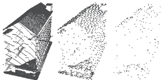
Fig. 5 Example of a point cloud of a building from the area of Brno. The original point cloud with the point density of 24 pt./ m^2 (left) and thinned point clouds with the density of 1.5 pt./ m^2 (middle) and 0.25 pt./ m^2 (right). Source: authors, graphical user interface of ArcInfo 10
