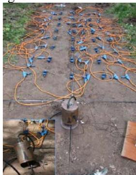
**Figure 1** Photo from the scene of the experiment. The inset shows the position of vibrator after the loss of soil's stability.
