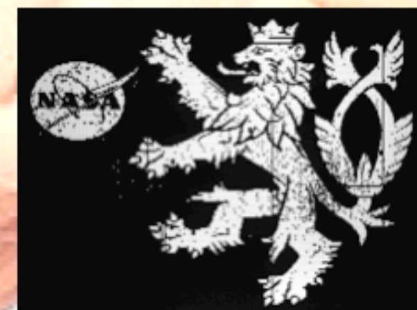
Image of Czech heraldic lion as a demonstration of 2D addressing by a microshutter array. The light pixels are open shutters, the dark pixels are closed shutters. It is possible that a blind patient with our proposed implant would see images with the same quality.
