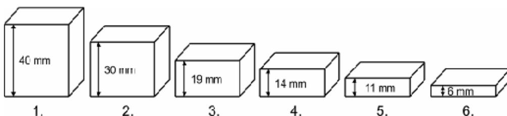
Figure 1. The specimens tested at pilot experimental investigations [8].
