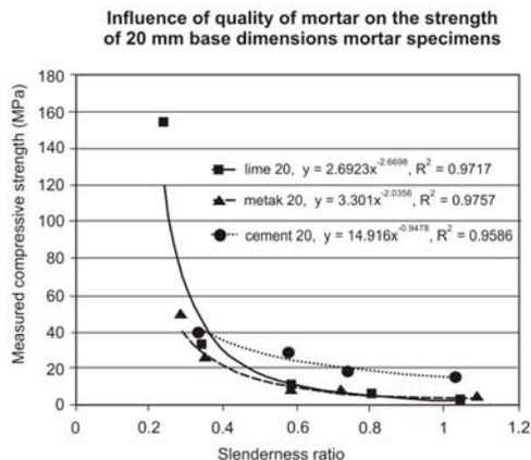
Figure 7. Dependence of the measured compressive strength to the standard strength ratio of specimens with the 20 mm base length on the slenderness and the standard strength (type of mortar).
