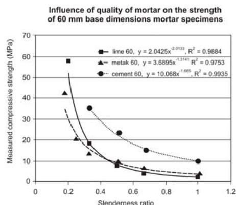
Figure 9. Dependence of the measured compressive strength to the standard strength ratio of specimens with the 60 mm base length on the slenderness and the standard strength (type of mortar).
