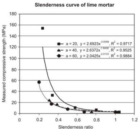
Figure 4. Dependence of the measured compressive strength of lime mortar on the slenderness and the base length.
