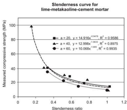
Figure 5. Dependence of the measured compressive strength of lime-metakaoline mortar on the slenderness and the base length.
