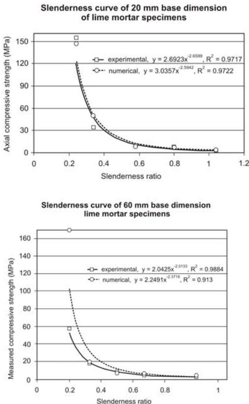
by the model compared with experimental results for all three base dimensions and different slenderness ratios. It is clear that even the simplified model chosen is capable of capturing the slenderness effect reasonably.
