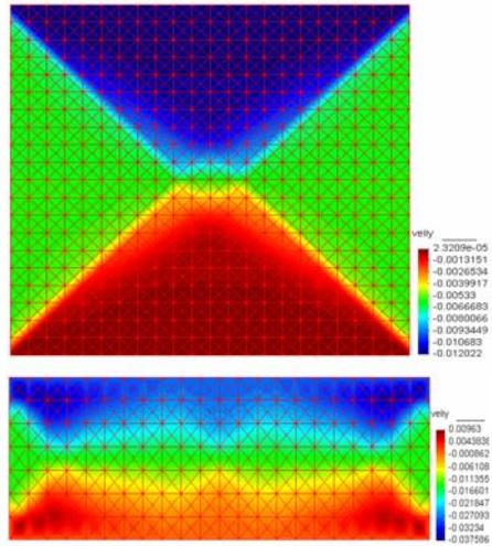
Figure 11. Vertical displacements for 40 mm base specimens of different slenderness ratios (heights of 40mm and 14 mm)
