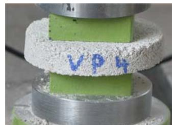
Figure 3. Concentrated compression tests on the round „cake-like“ specimen.
