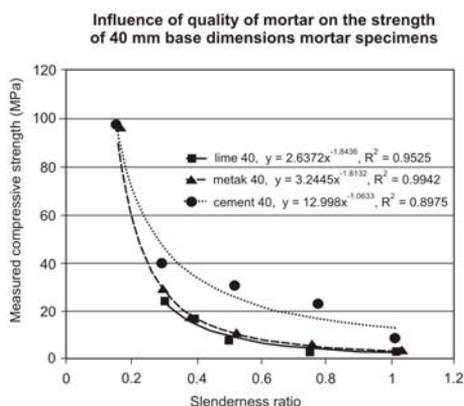
Figure 8. Dependence of the measured compressive strength to the standard strength ratio of specimens with the 40 mm base length on the slenderness and the standard strength (type of mortar).
