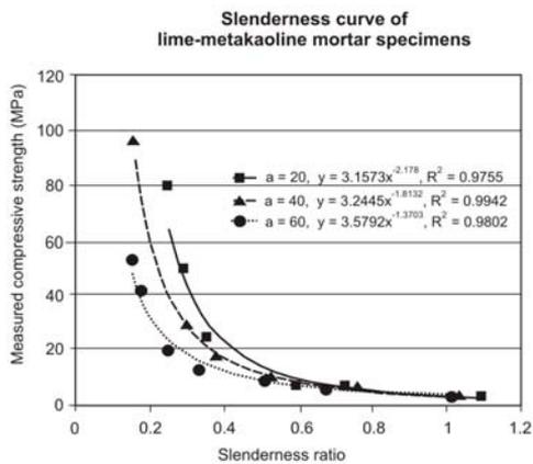
Figure 6. Dependence of the measured compressive strength of lime-metakaoline-portland cement mortar on the slenderness and the base length.
