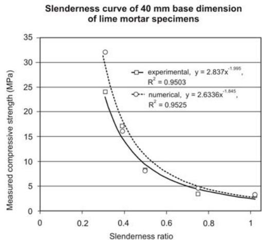
Figure 12. Comparison of computed and measured compressive strengths.
