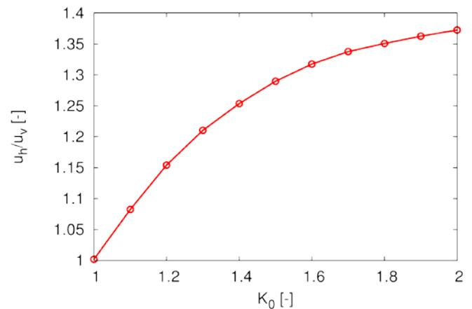
Figure 9. Dependency of the ratio of  $u_h/u_v$  on the value of  $K_0$  obtained in 2D analyses for constant value of the factor  $\lambda_2=0.67$ .
