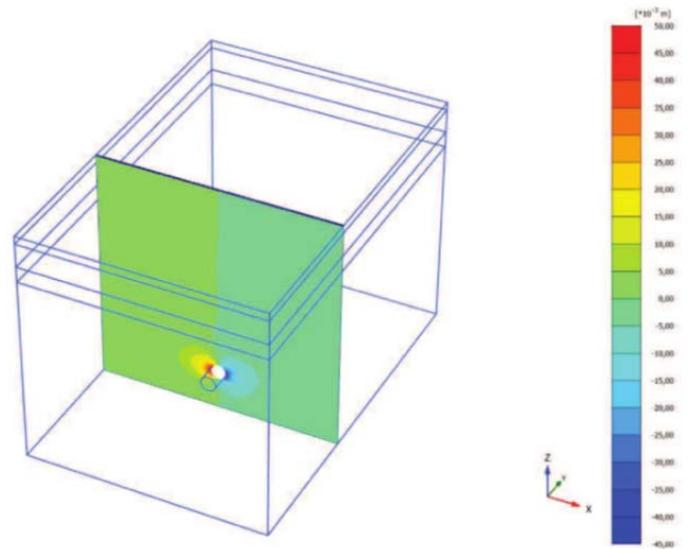
Figure 8. 3D model geometry and predictions of horizontal displacements.
