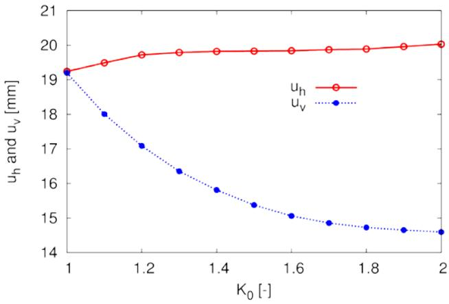
Figure 10. Dependency of the ratio of  $u_h/u_v$  on the value of  $K_0$  obtained in 2D analyses for constant value of the factor  $\lambda_2=0.67$ .
