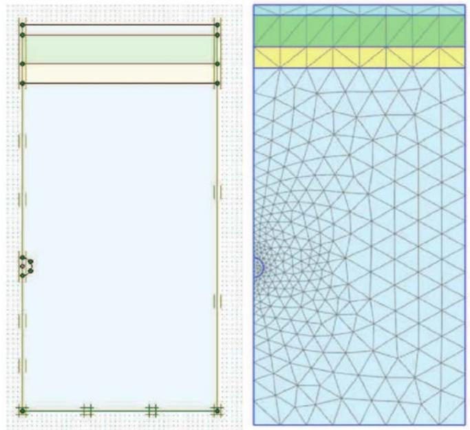
Figure 5. Geometry of 2D numerical model of the circular adit
