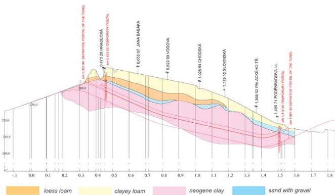
Figure 2. Longitudinal geological cross-section at the site of Dobrovského tunnels (Pavlík et al., 2004).
