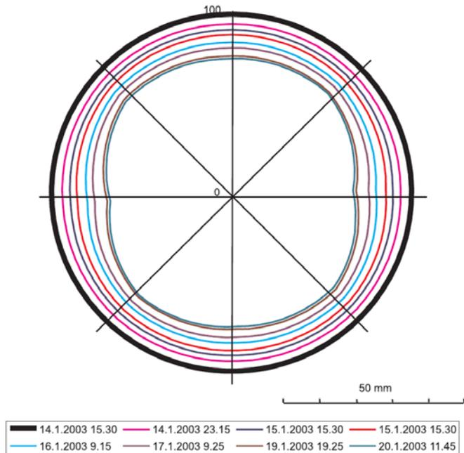
Figure 5. Results of the convergence measurement of the circular adit R2 (Pavlík et al., 2004).
