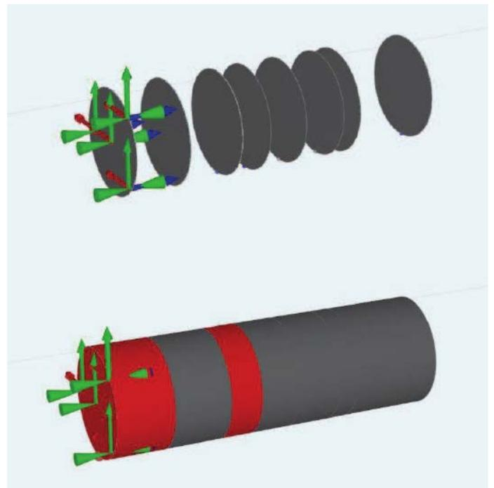
Figure 6. Detail of the geometry of 3D numerical model of the circular adit
