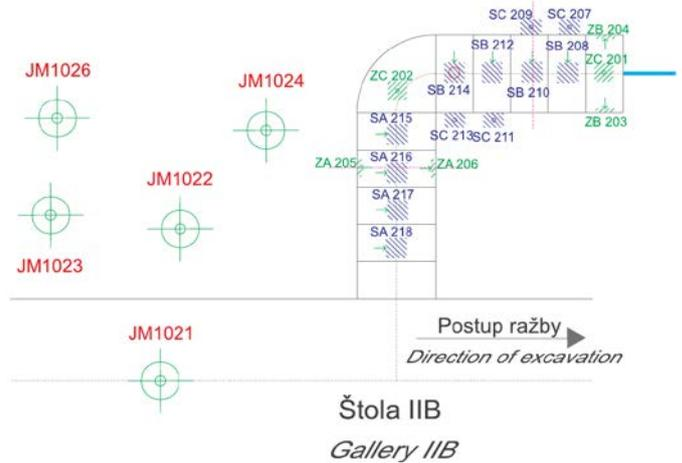
Figure 3. Geometry of the circular exploratory adit R2 excavated from the Gallery IIB (Pavlík et al., 2004).
