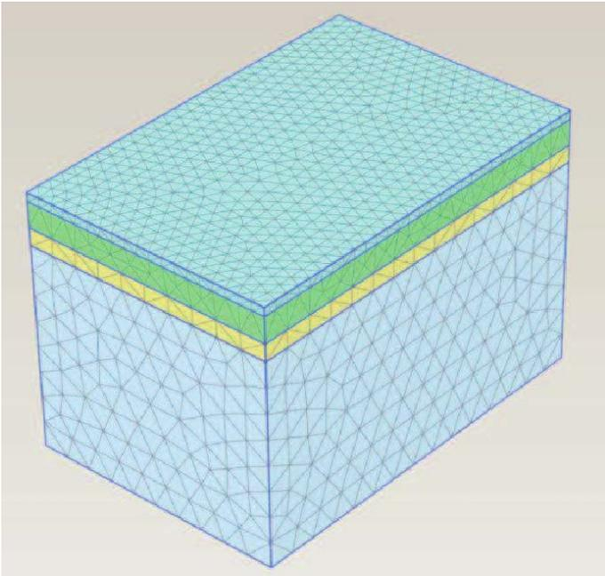
Figure 7. Simulated domain of the 3D numerical model of the circular adit
