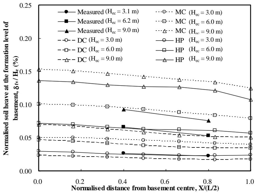
**Fig. 5. A comparison of the measured and computed basement heave.**
