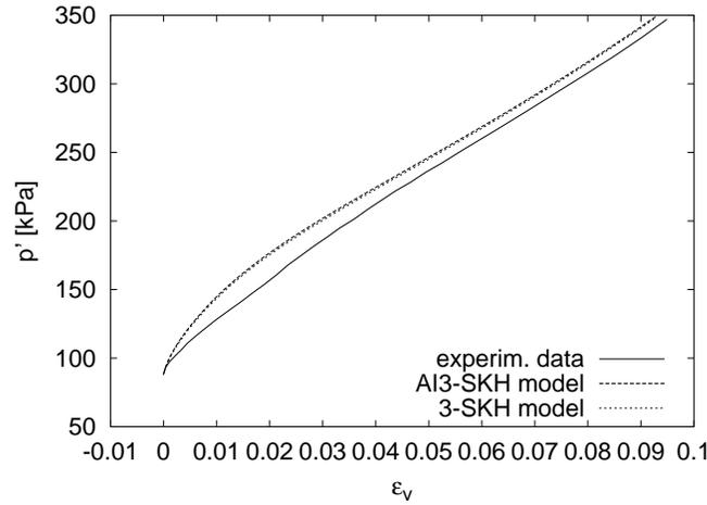
**Figure 6.**  $p'/\epsilon_v$  results of the test R0 (test data after Callisto, 1996) and simulations by the 3-SKH and AI3-SKH model.
