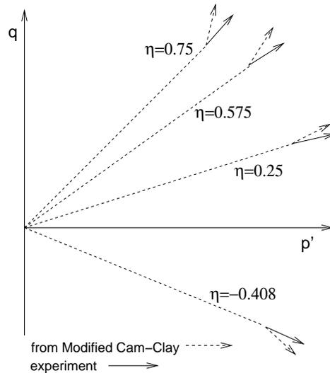
**Figure 2.** Values of the total strain increment ratio predicted from the Modified Cam–Clay model and observed during anisotropic compression for reconstituted London Clay (after Richardson, 1988)
