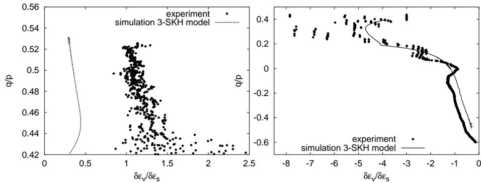
**Figure 3.**  $\delta\epsilon_v/\delta\epsilon_s - q/p$  plots for tests on reconstituted Pisa Clay (test data from Callisto, 1996) R30 (left) and R315 (right) and simulation by the 3-SKH model.
