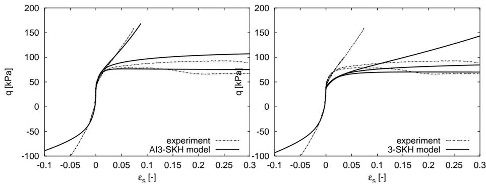
**Figure 5.**  $q/\epsilon_s$  plots for tests on reconstituted Pisa Clay (test data after Callisto, 1996). Simulations with the AI3-SKH model (left) and 3-SKH model (right).
