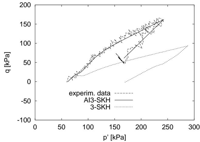
**Figure 4.** Stress path of the  $K_0$  loading and unloading test on Boom Clay (test data after Coop et al. (1995)) and simulation by the AI3-SKH and 3-SKH model.
