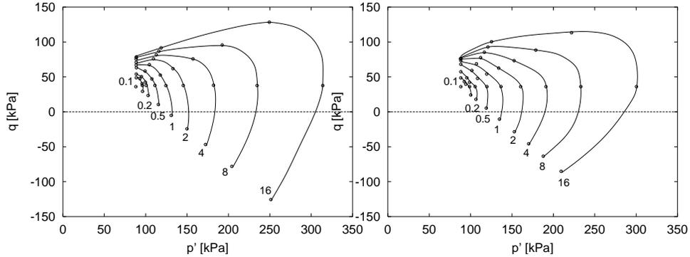
**Figure 8.** Contours of the equal specific strain energy (in  $\text{kJ}/\text{m}^3$ ), experimental data (after Callisto, 1996) (left) and simulations by the AI3-SKH model (right)
