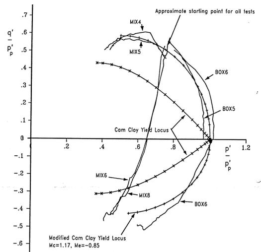
**Figure 1.** Stress paths for  $K_0$  normally compressed samples normalized with respect to specific volume (Pickles, 1989) Tests MIX4, MIX5, BOX5 and BOX6 direction toward state boundary surface, MIX6 and MIX8 undrained unloading
