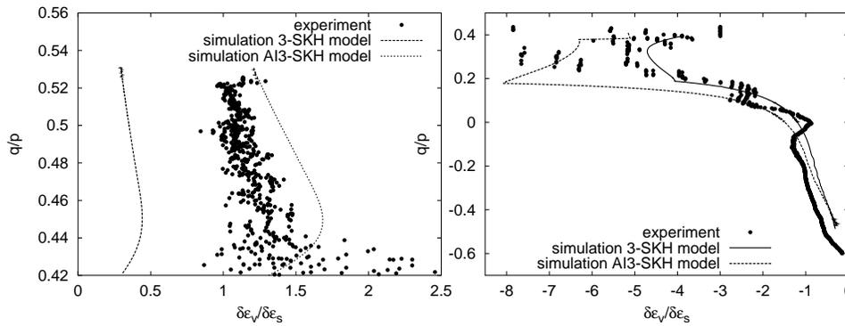
**Figure 7.**  $\delta\epsilon_v/\delta\epsilon_s - q/p$  plots for tests on reconstituted Pisa Clay (test data from Callisto, 1996) R30 (left) and R315 (right) and simulation by the 3-SKH model and AI3-SKH model.
