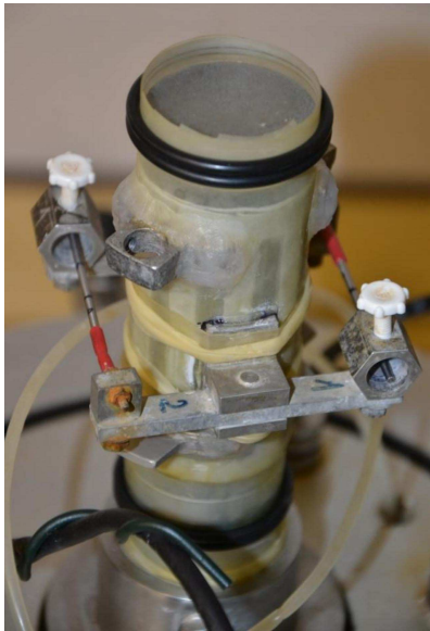
Figure 8: Setup for local LVDT measurements of radial and axial strain (LVDTs not mounted for clarity of the photograph).
