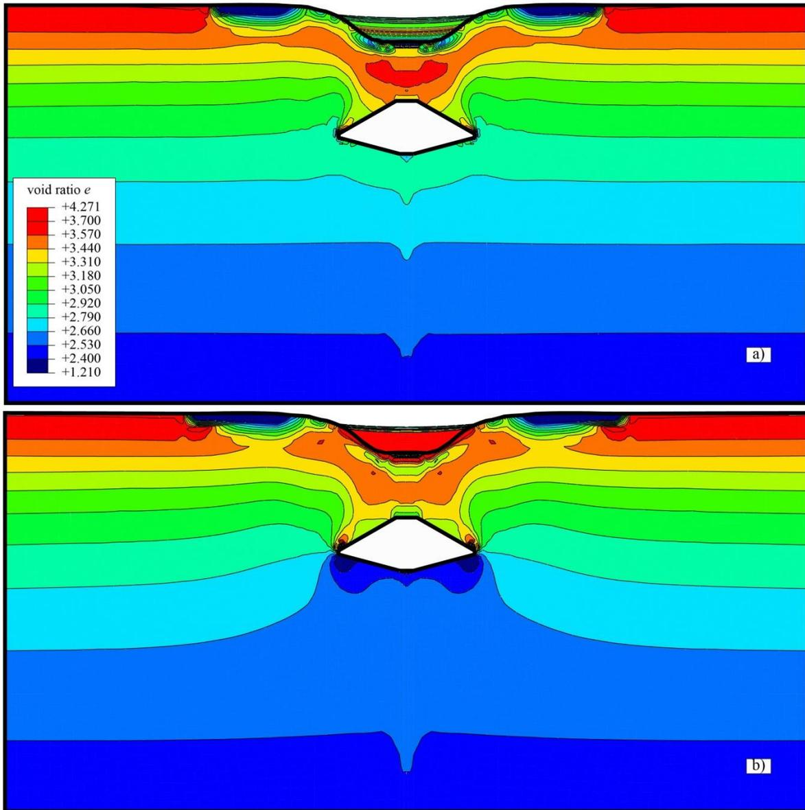
Figure 12: Void ratio distribution a) without consolidation and b) with consolidation  $T = 0.05$
