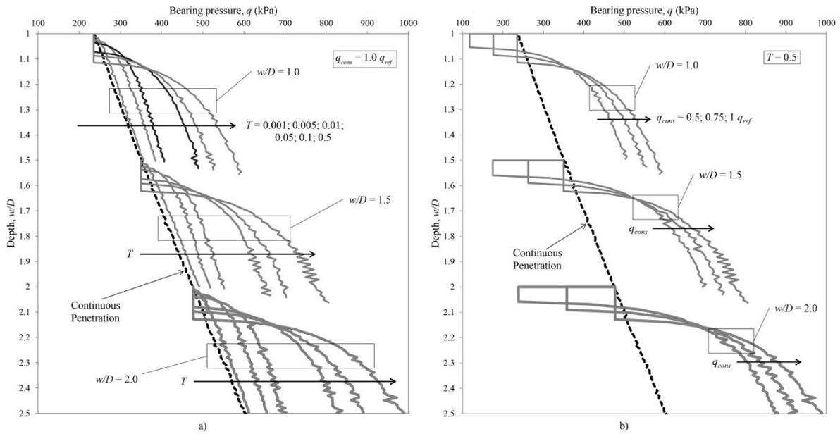
Figure 6: Load-penetration curves at increasing depth  $w/D = 1.0; 1.5; 2$  showing the effects on further spudcan penetration of different a) length of consolidation  $T = 0.001; 0.005; 0.01; 0.05; 0.1; 0.5$  at constant  $q_{cons}/q_{ref} = 1$  and b) fraction of load held in consolidation  $q_{cons}/q_{ref} = 0.5; 0.75; 1.0$  at constant  $T = 0.5$
