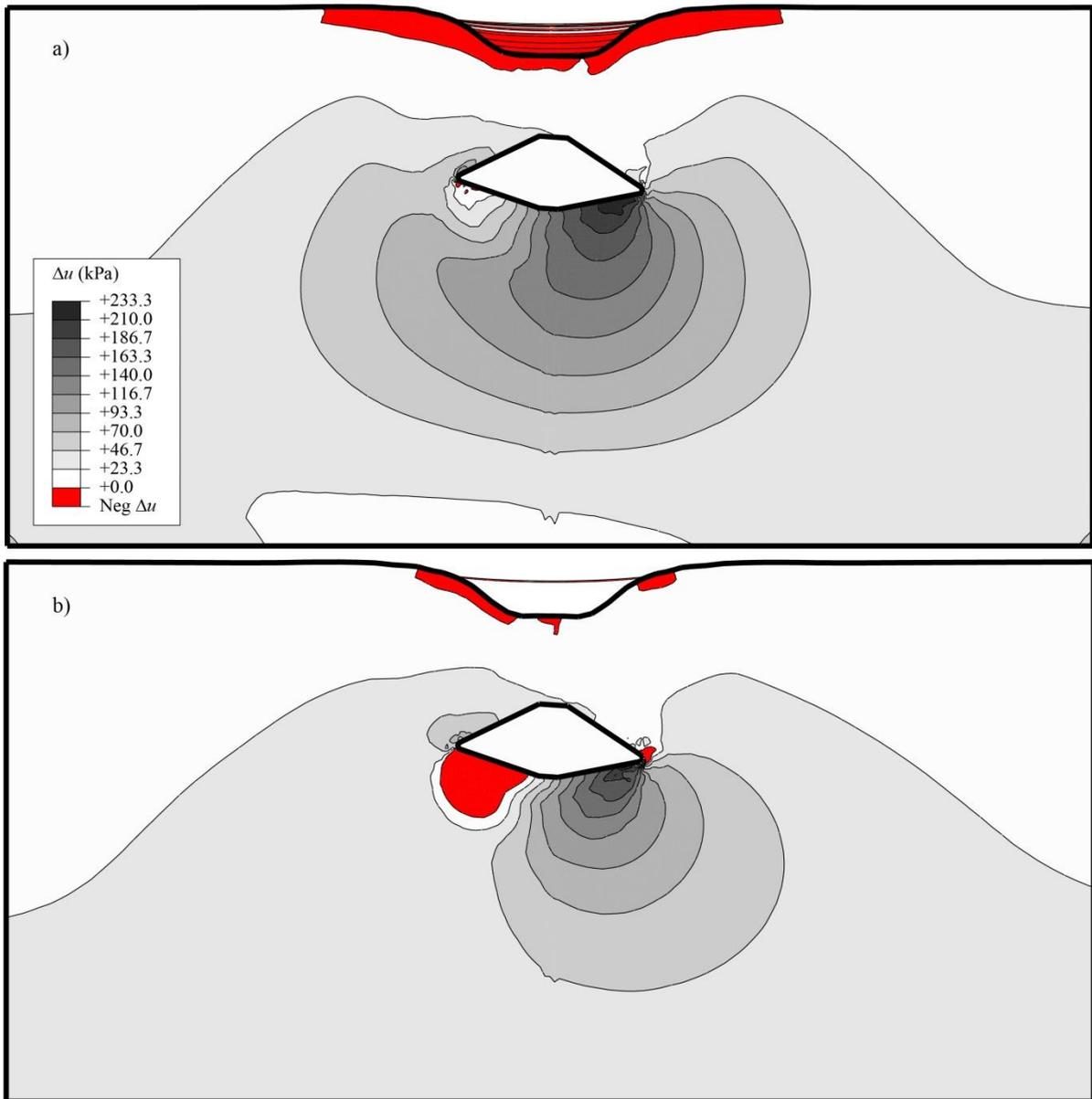
Figure 14: Comparison of excess pore pressure contours following pure rotation a) without consolidation  $T = 0$ ; b) including a period of consolidation  $T = 0.05$
