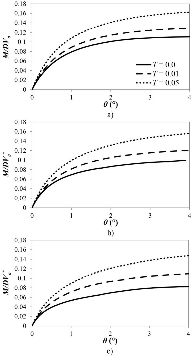
Figure 9: Moment-rotation curves ( $\theta - M/DV_0$ ) following pure rotation at increasing  $T$  for a)
