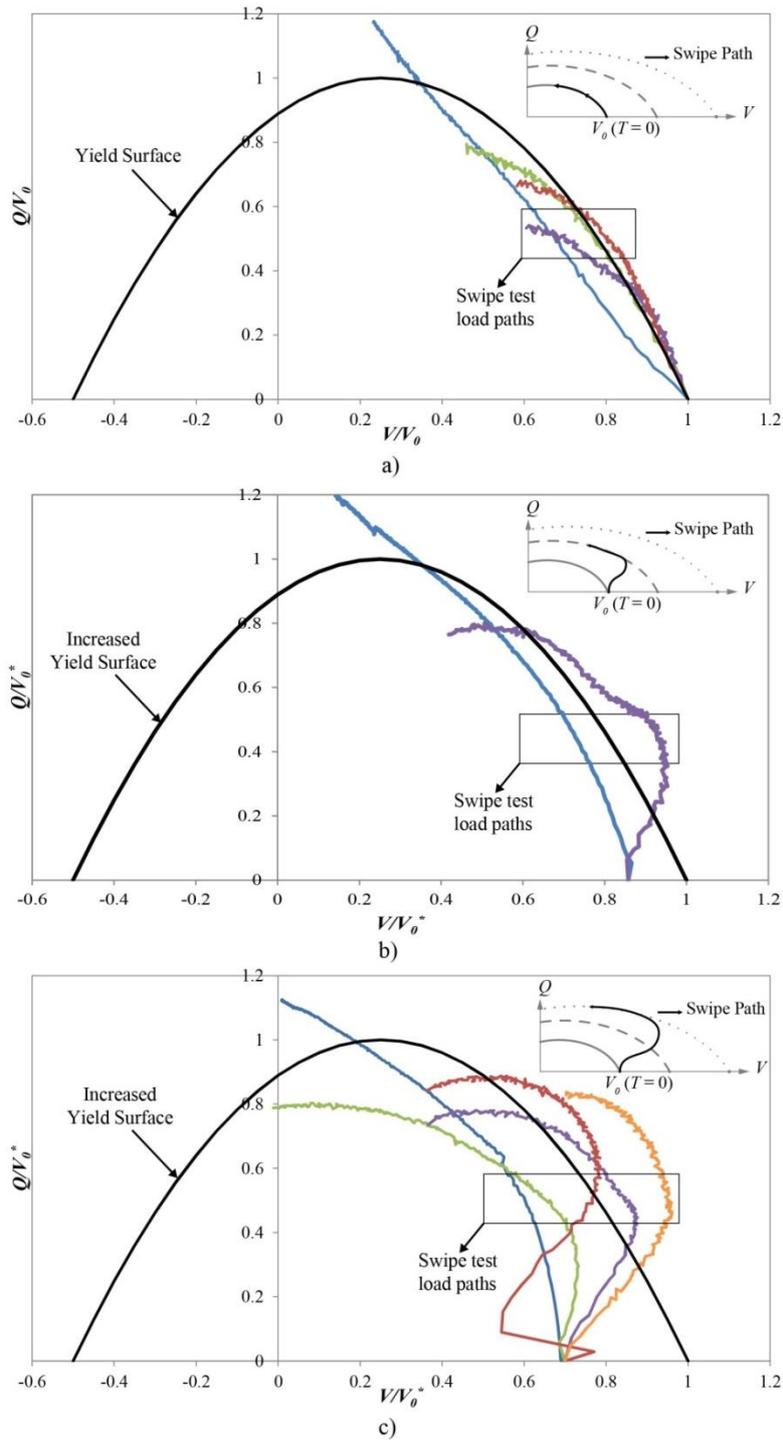
Figure 17: Results from experimental swipe tests in the normalised  $Q/V_0$ - $V/V_0$  plane for increasing consolidation a)  $T = 0$ ; b)  $T = 0.01$ ; c)  $T = 0.05$
