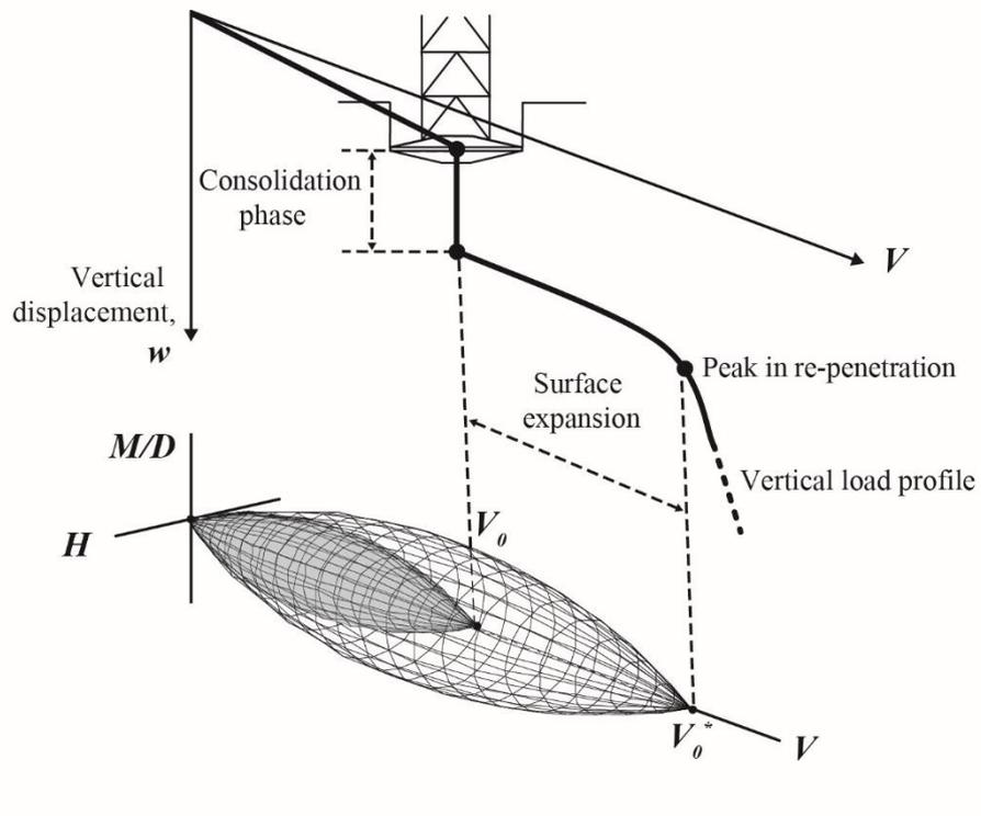
Figure 1: Three dimensional yield surface and its expansion due to consolidation
