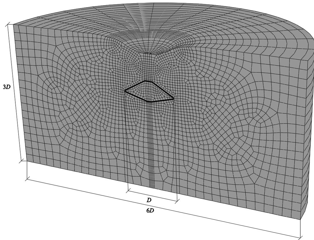
Figure 4: Mesh density and soil domain dimensions
