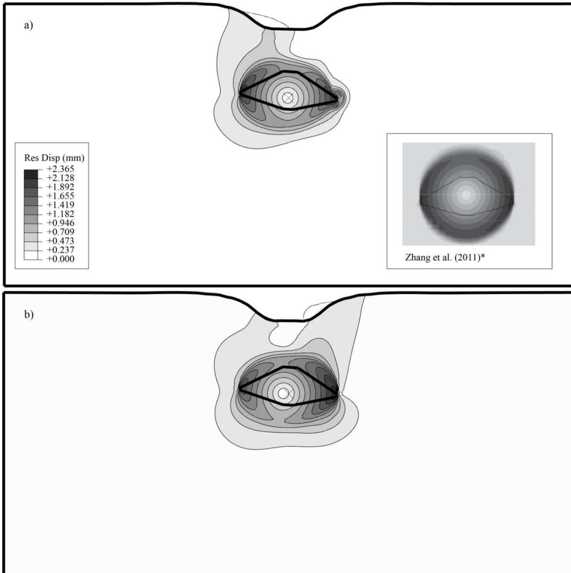
Figure 11: Comparison of resultant displacement contours following pure rotation a) without consolidation  $T = 0$ ; b) including a period of consolidation  $T = 0.05$
