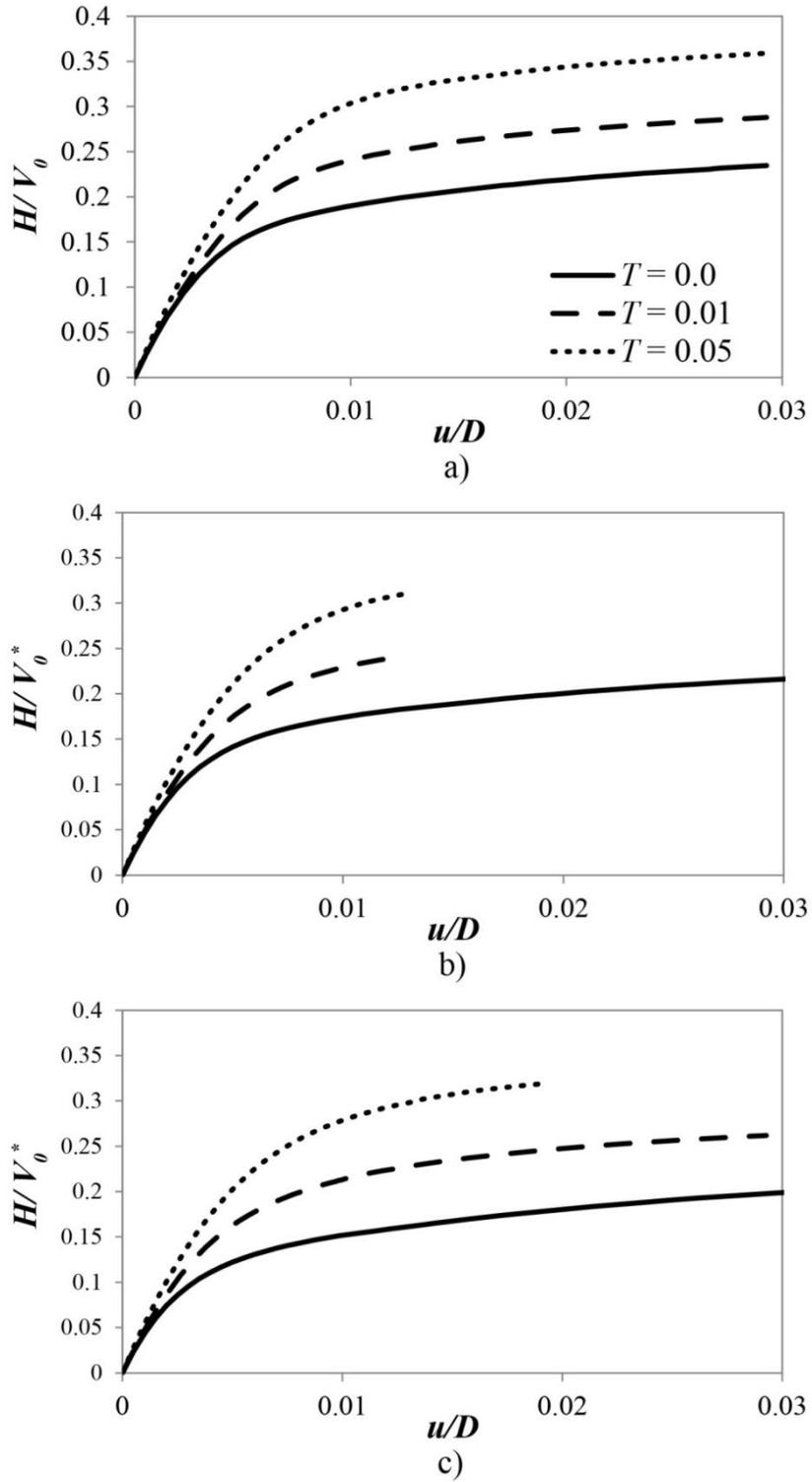
Figure 8: Load-displacement curves ( $u/D - H/V_0$ ) following pure horizontal displacement at increasing  $T$  for a)  $V = 0.5V_0$  ( $T = 0$ ); b)  $V = 0.75V_0$  ( $T = 0$ ); c)  $V = 0.9V_0$  ( $T = 0$ )
