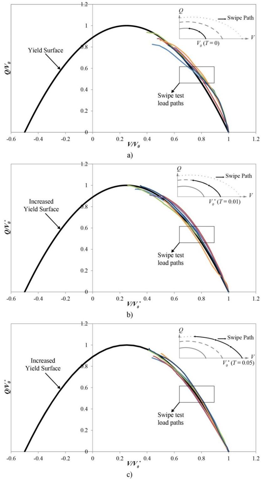
Figure 15: Results from numerical simulation of swipe tests in the normalised  $Q/V_0$ - $V/V_0$  plane for increasing consolidation a)  $T = 0$ ; b)  $T = 0.01$ ; c)  $T = 0.05$
