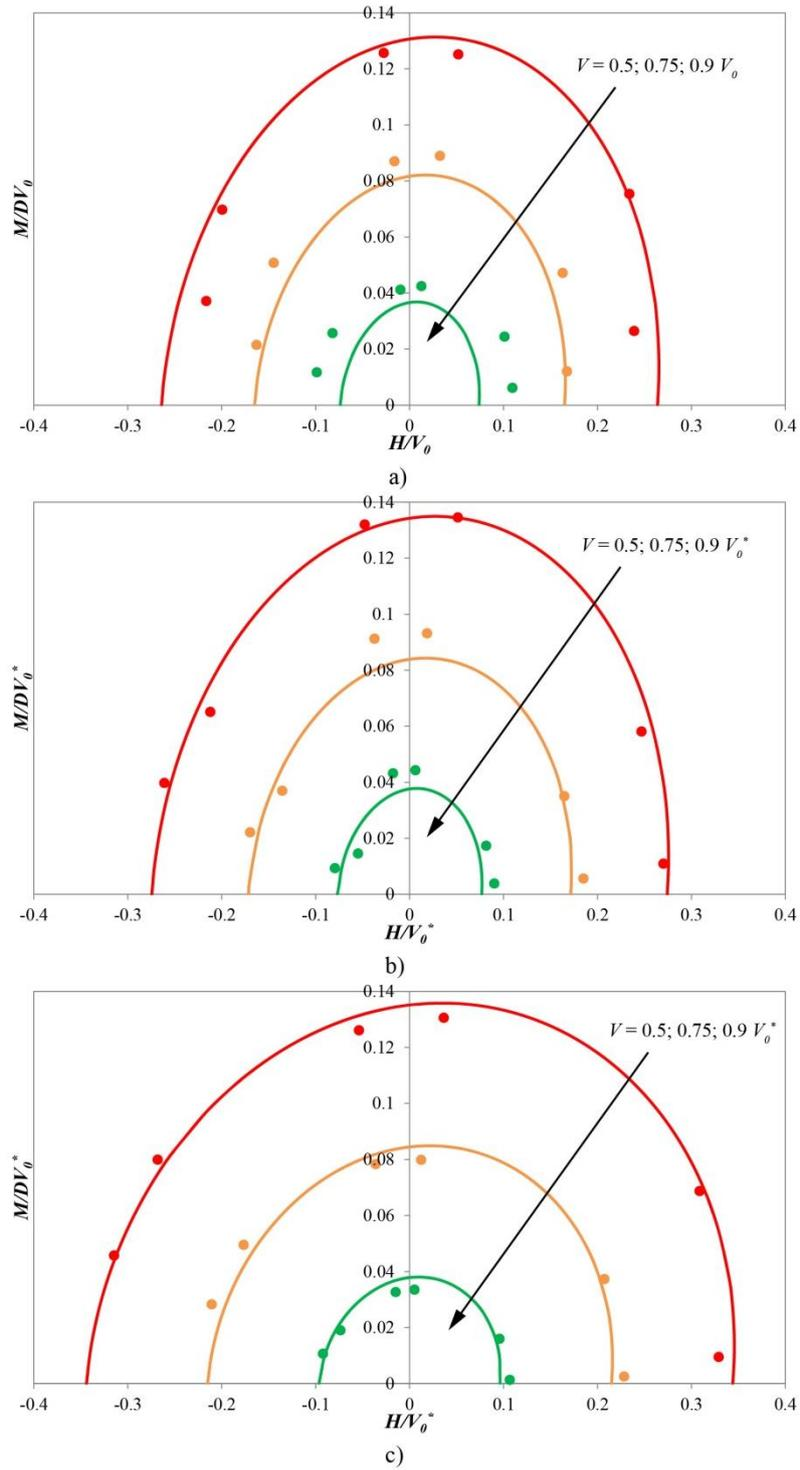
Figure 16: Sections of the yield surfaces obtained with numerical simulation in the normalised  $H/V_0$ - $M/DV_0$  plane for increasing  $V = 0.5; 0.75; 0.9 V_0$  (or  $V_0^*$ ) and consolidation
