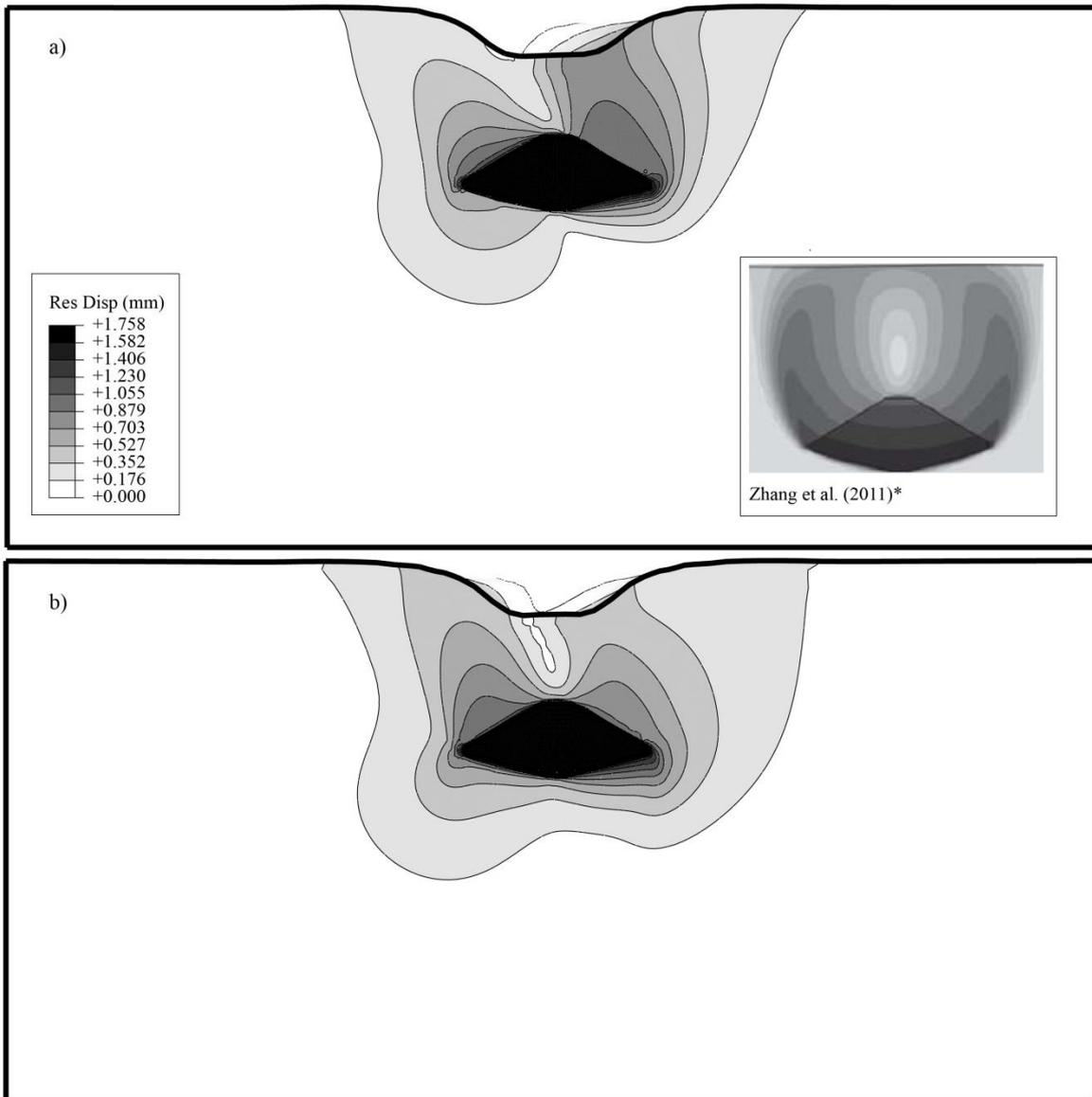
Figure 10: Comparison of resultant displacement contours following pure horizontal displacement a) without consolidation  $T = 0$ ; b) including a period of consolidation  $T = 0.05$ .
