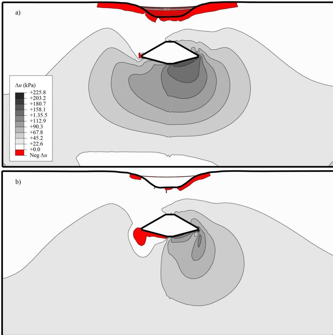
Figure 13: Comparison of excess pore pressure contours following pure horizontal displacement a) without consolidation  $T = 0$ ; b) including a period of consolidation  $T = 0.05$
