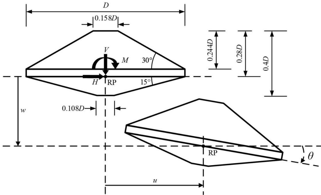
Figure 3: Spudcan geometry and load-displacement convention
