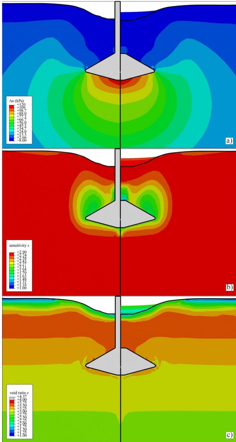
Figure 5: Results of mapping a) excess pore pressure; b) sensitivity; c) void ratio; from two- (LHS) to three-dimensional (RHS) analyses
