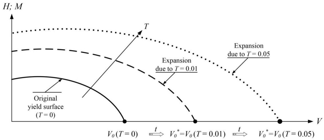
Figure 7: Schematic of increase in yield surface size and  $V_0$  magnitude due to a period of consolidation
