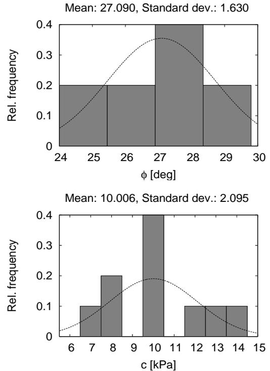
Figure 4. Statistical distributions of  $\varphi$  and  $c$  as measured by Sevaldson (1956)
