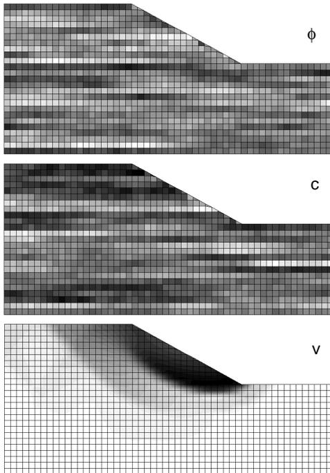
Figure 6. Typical realisation of random fields of uncorrelated variables  $\varphi$  and  $c$  for  $\theta_h = 100$  m and  $\theta_v = 1$  m, together with the velocity field at failure. Lighter areas of  $\varphi$  and  $c$  are softer.
