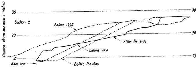
Figure 2. Mid-section through the Lodalen slide, from Sevaldson (1956)
