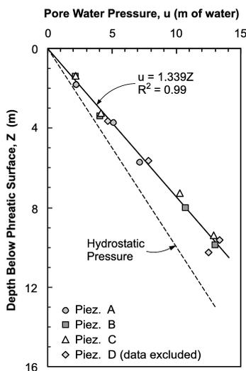
Figure 3. Pore pressures measured at the Lodalen site (El-Ramly et al., 2006; data from Sevaldson, 1956)
