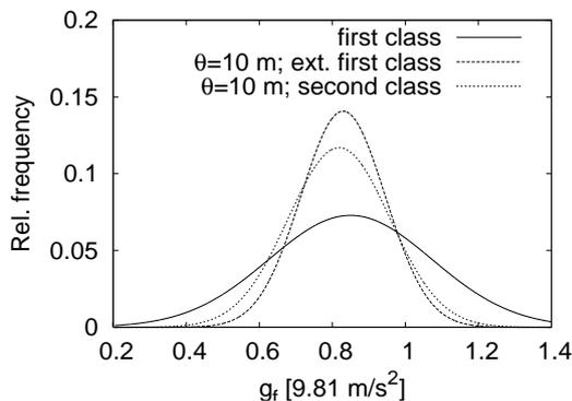
Figure 9. Distributions of  $g_f$  for the first class, extended first class, and second class methods for  $\theta = 10$  m.
