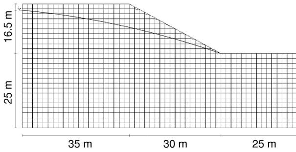
Figure 5. Finite element mesh used, with dimensions and assumed position of the ground water table.
