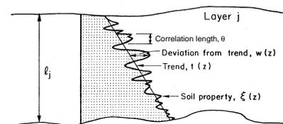
Figure 1. Characterisation of inherent soil variability (after Phoon and Kulhawy 1999, modified).
