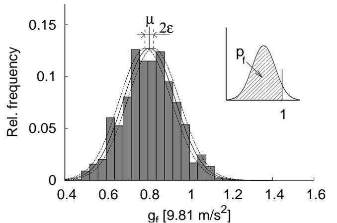
Figure 7. Evaluation of the probability of failure and 95.4 % confidence intervals of the Monte Carlo simulation from the statistical distribution of the gravity acceleration at failure  $g_f$  for the case  $\theta_h = \theta_v = 10$  m.
