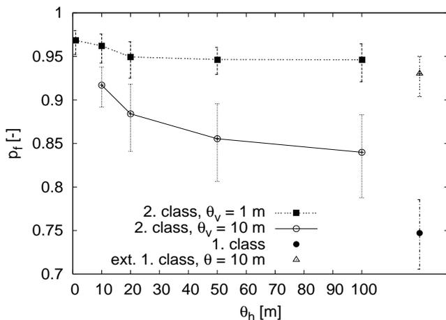
Figure 8. Probability of failure as a function of the correlation length. Results by the first class and extended first class methods included.
