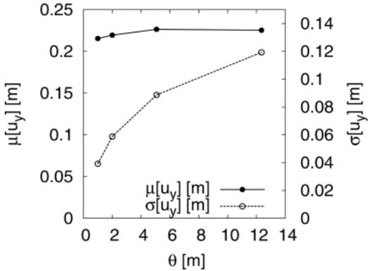
Figure 11. The dependency of  $\mu[u_y]$  and  $\sigma[u_y]$  on  $\theta_v$  predicted by the random field method.
