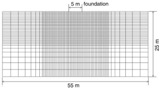
Figure 5. The problem geometry and finite element mesh.
