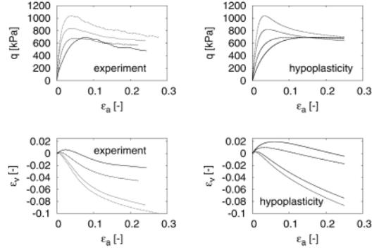
Figure 2. Typical experimental and simulated results of drained triaxial tests.
