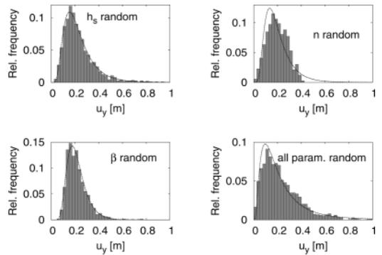
Figure 8. Probabilistic distributions of  $u_y$  for Monte-Carlo analyses with infinite correlation length.
