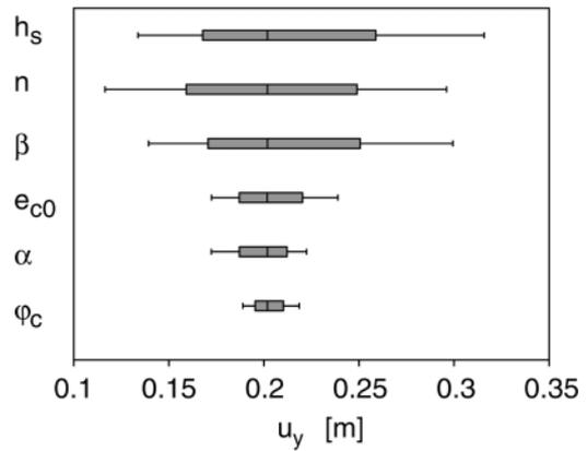
Figure 6. Tornado diagram showing sensitivity of foundation displacements on different parameters.
