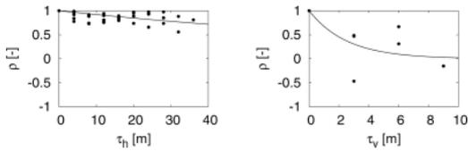
Figure 4. Evaluation of the correlation coefficient  $\rho$  in horizontal (a) and vertical (b) directions for parameter  $\phi_c$ , together with least square fit of Eq. (1).
