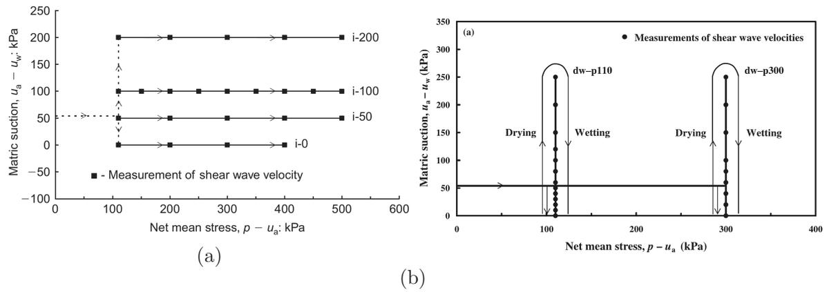
Figure 2: (a) Stress-suction paths of simulated isotropic compression tests [37]; (b) Stress-suction paths of simulated wetting-drying tests [36].
