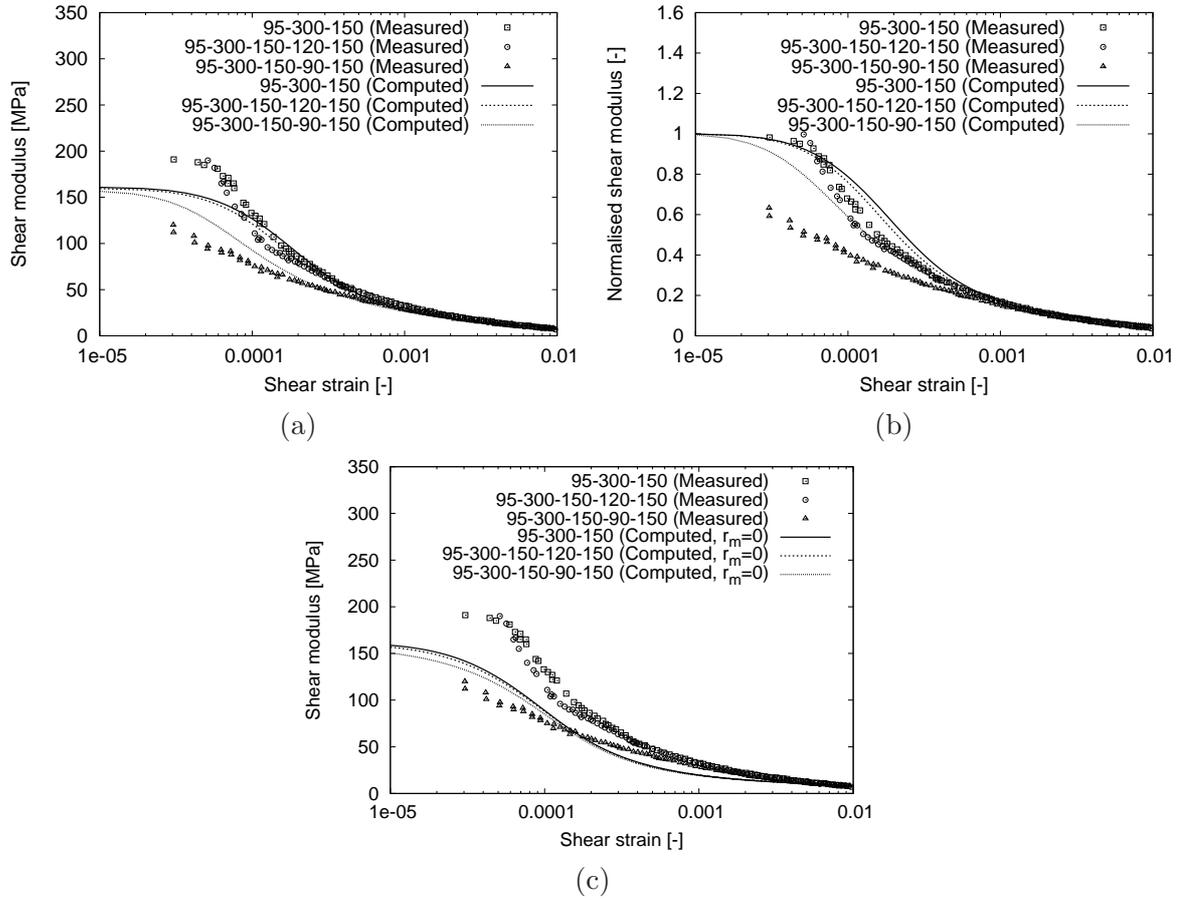
Figure 11: Simulations of the fourth set of experiments. (a) Stiffness degradation curves, (b)  $G/G_{tp0}$  vs. shear strain curves, (c) stiffness degradation curves simulated with  $r_m = 0$ . Experimental data by Ng and Xu (2012) compared with the model predictions.
