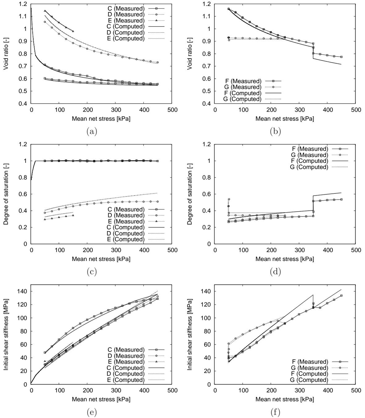
Figure 14: Simulations of Zenos Kaolin experiments, constant suction paths. Experimental data by Biglari et al. (2012).
