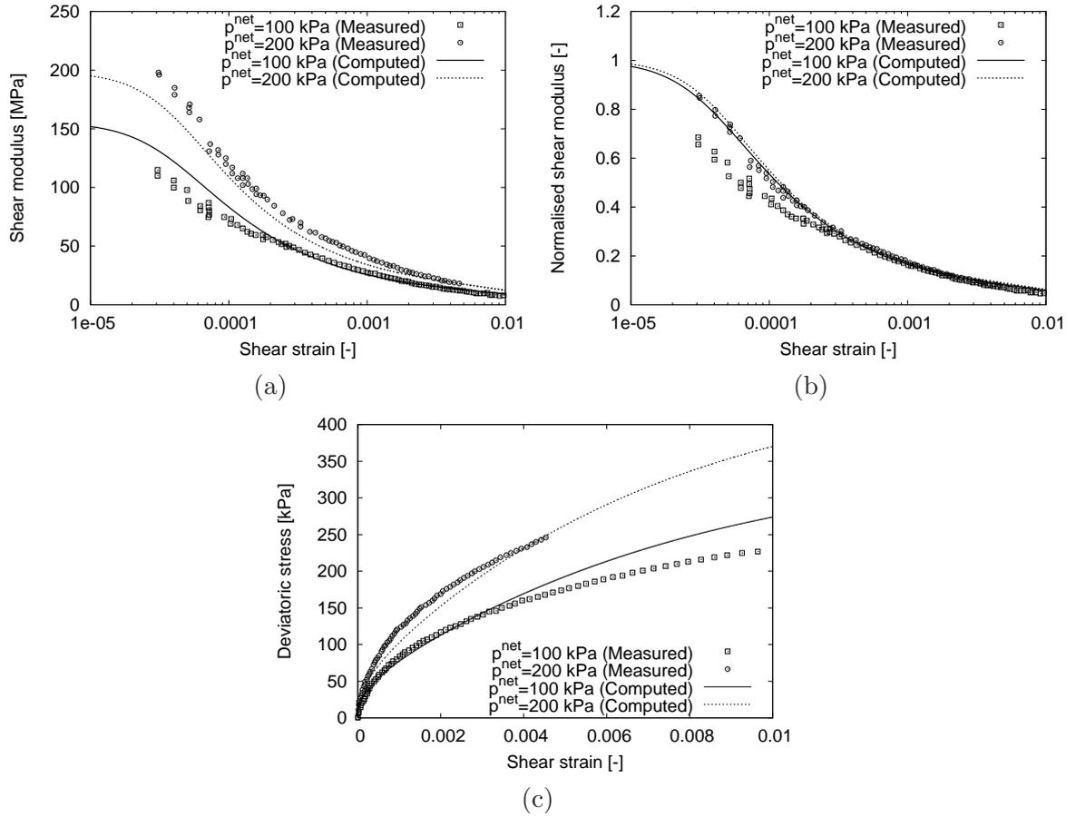
Figure 12: Simulations of the fifth set of experiments, experimental data by Ng and Xu (2012) compared with the model predictions. (a)  $G$  vs. shear strain curve, (b)  $G/G_{tp0}$  vs. shear strain curve, (c) deviatoric stress vs. shear strain curve
