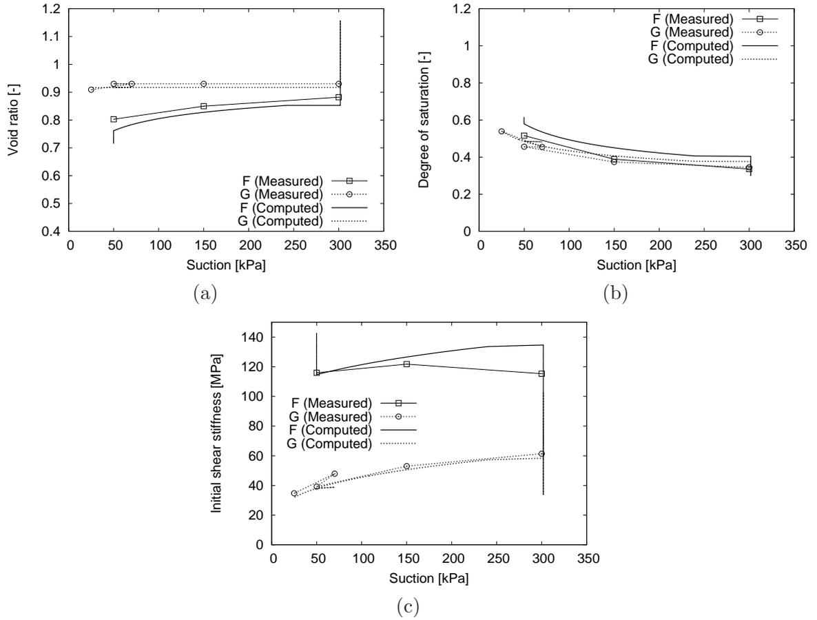
Figure 15: Simulations of Zenos Kaolin experiments, constant  $p^{net}$  paths. Experimental data by Biglari et al. (2012).
