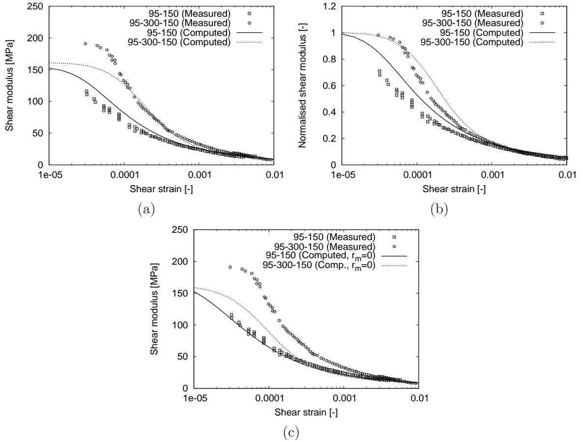
Figure 9: Simulations of the second set of experiments. (a) Stiffness degradation curves, (b)  $G/G_{tp0}$  vs. shear strain curves, (c) predictions with  $r_m = 0$ . Experimental data by Ng and Xu (2012) compared with the model predictions.
