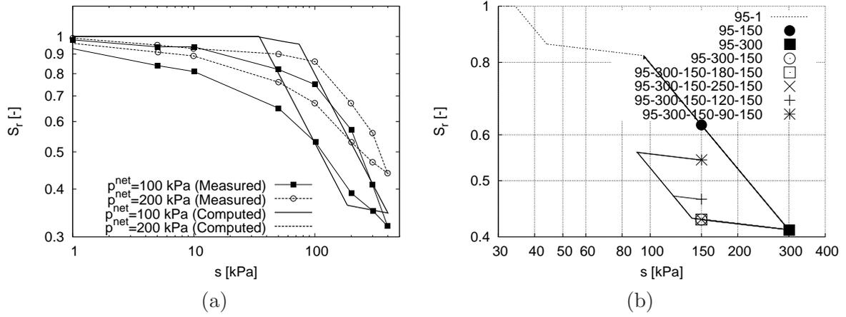
Figure 6: Hysteretic water retention curve. (a) Experimental data by Ng and Xu (2012) and model predictions. (b) Suction vs  $S_r$  histories and initial hydraulic states of the simulated shear tests.
