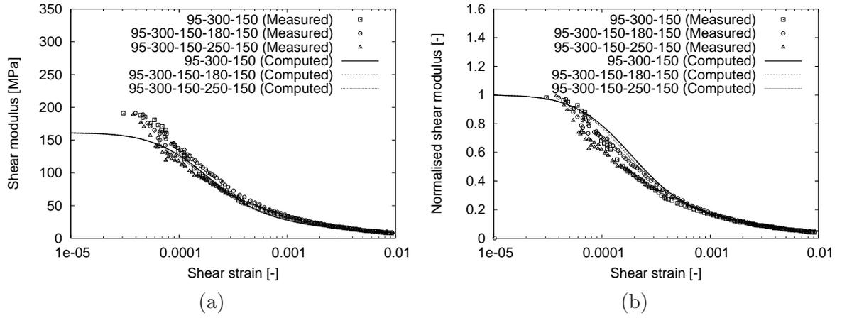
Figure 10: Simulations of the third set of experiments. (a) Stiffness degradation curves, (b)  $G/G_{tp0}$  vs. shear strain curves. Experimental data by Ng and Xu (2012) compared with the model predictions.
