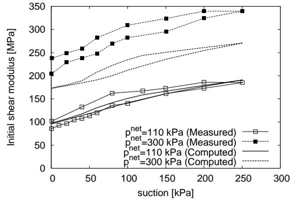
Figure 4:  $G_{tp0}$  dependency on suction during constant mean net stress wetting-drying tests. Experimental data by Ng et al. [36] and model simulations.
