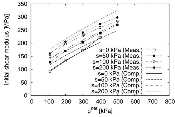
Figure 3:  $G_{tp0}$  dependency on mean net stress during constant suction isotropic compression tests, experimental data by Ng and Yung [37] and model simulations.
