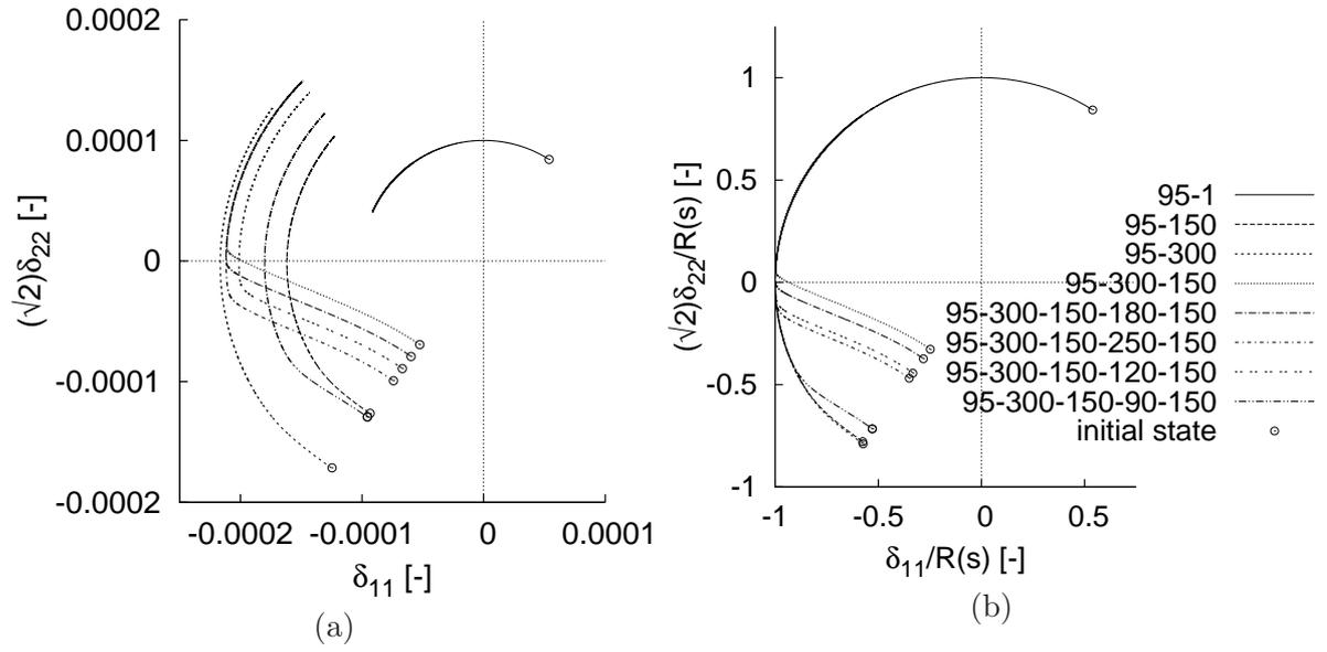
Figure 7: Intergranular strain evolution during the shear phase in different tests at  $p^{net} = 100$  kPa. (a) vertical ( $\delta_{11}$ ) and horizontal ( $\delta_{22}$ ) components of the intergranular strain; (b) intergranular strain normalised by  $R(s)$ . 95 – 300 – 150 – 50 – 150 is identical to 95 – 300 – 150 – 90 – 150 and not shown for clarity.
