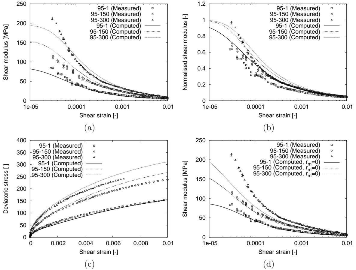
Figure 8: Stiffness degradation curves from the first set of experiments, experimental data by Ng and Xu (2012) compared with the model predictions. (a)  $G$  vs. shear strain curve, (b)  $G/G_{tp0}$  vs. shear strain curve, (c) deviatoric stress vs. shear strain curve, (d)  $G$  vs. shear strain curve predicted by the model with  $r_m = 0$ .
