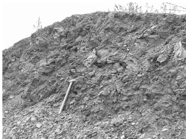
Figure 2. Material of the landfill after about ten years from filling (landfill "Pokrok" near the town of Bilina, North Bohemia).
