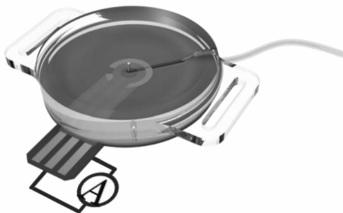
Fig. 1 The flow-through glucose or lactate biosensor.
