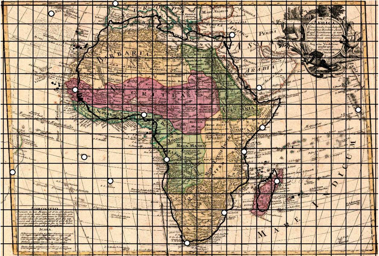
Figure 1: Georeferencing of a small-scale early map in the Bonne projection to the Mercator projection using the similarity transformation; the transformation key is determined from the identical points.
